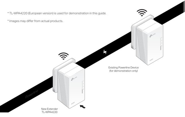
Plug in the new extender near one of your existing powerline devices.
