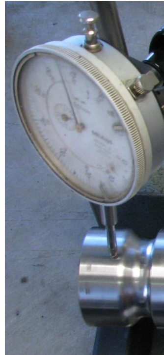
Figure 49 – Dial Indicator Position for Crankshaft & Prop Flange Run Out
