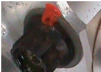
Figure 13 - Torque seal installed
