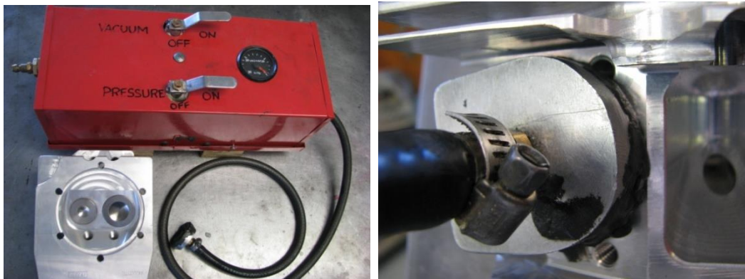
Figure 18 – Valve Leakage Vacuum Tester
