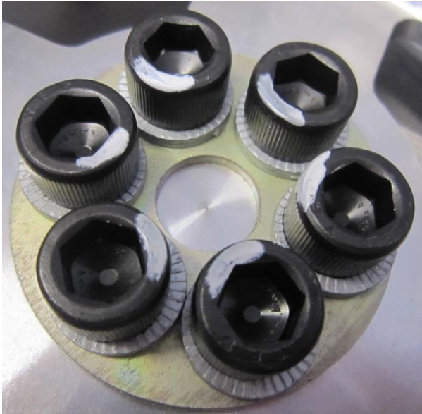
Figure 46: Flywheel bolts installed with Nordlocs and steel wear plate.
