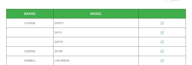
We highly recommend using an LED dimmer that is also an ELV (electronic low voltage) dimmer. A buzzing or flickering light is typically an indication that the dimmer being used is not compatible with the lights. Please consult dimmer manufacturer for maximum lamps per dimmer capacity.
