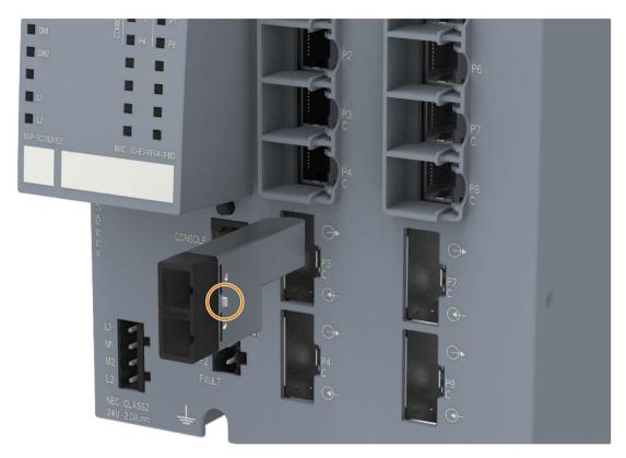
Figure 4-2 Inserting an SCP / STP transceiver
