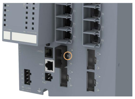
Figure 5-1 Removing an SCP / STP transceiver
