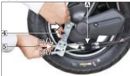
(4) Integrated brake arm (5) First adjuster nut (i) Decrease free play (ii) Increase free play
