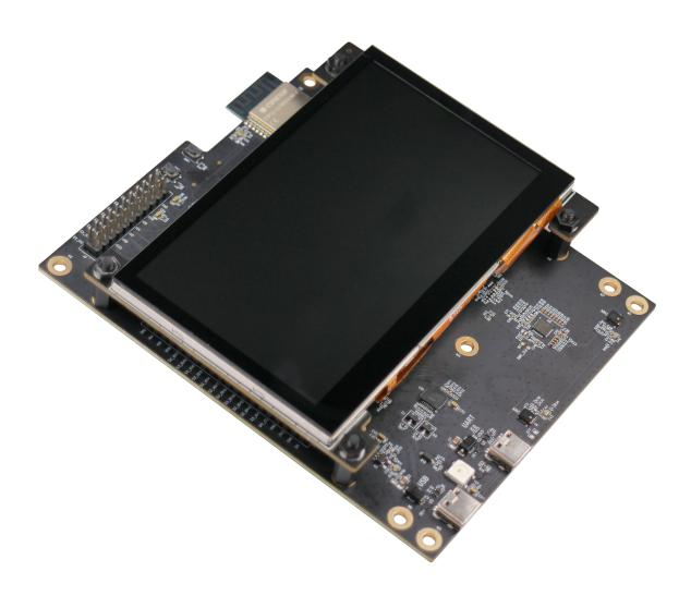
Fig. 27: ESP32-S3-LCD-Ev-Board with ESP32-S3-WROOM-1 Module
