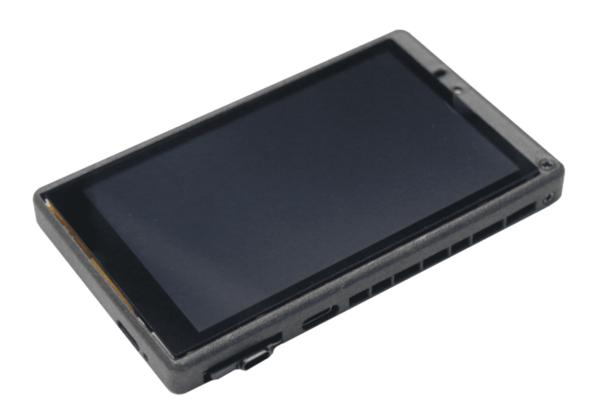
Fig. 58: ESP32-S2-HMI-DevKit-1 with ESP32-S2-WROVER module
