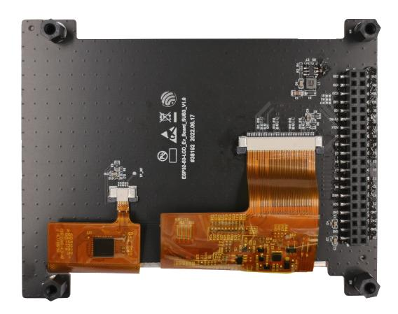
Fig. 33: ESP32-S3-LCD-Ev-Board\_SUB3 - Back (Click to Enlarge)
