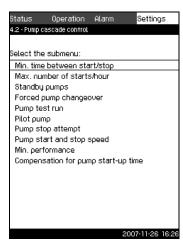
Fig. 48 Pump cascade control
