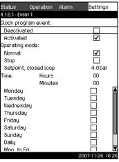
5. Mark operating mode **Normal** or **Stop** with  $\bigcirc$  or  $\bigcirc$ , and press  $\bigcirc$  (If **Stop** is selected, point 7 is skipped.)
