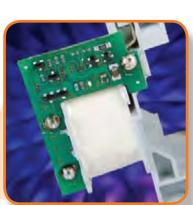
24V DC Electronic Coil with integrated (built-in) diode
