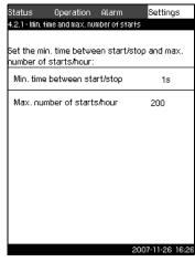
Fig. 49 Min. time between start/stop
