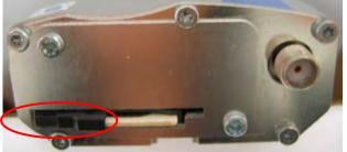
SIM card is inserted and being locked properly. GSM network is ready for use.
