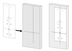
NOTE: Drill from both sides to avoid splintering the finished surface of wood doors. Not all holes are thru.
