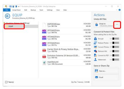
Choose the MicroSD memory device as the location to which to extract the folder from the zip file. This will create a new EQUIP folder, or over-write the existing EQUIP folder and any files contained within it. Click Unzip.
