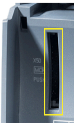
Figure 3-1 Slot for the SD card (yellow frame)
