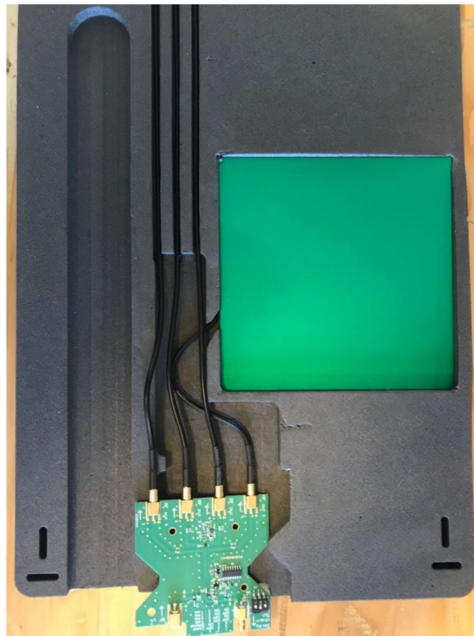
Figure 10 : Cluster 4 antennas fitted with Circular Patch Antennas
