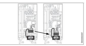
Reposition the mains terminal further downwards. To do this, undo the fixing screw. Secure the mains terminal in place.
