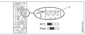
1 Jumper for anti-scalding protection setting
