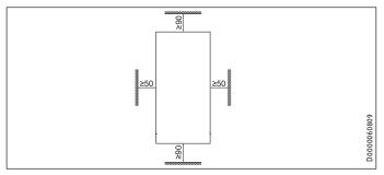
Maintain the minimum clearances to ensure trouble-free operation of the appliance and facilitate maintenance work.
