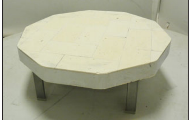
The Kiln Base positioned on the Stand:
