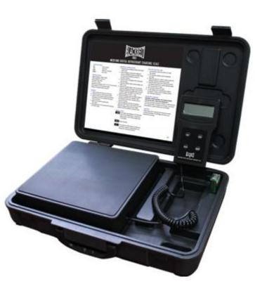
Carrier ductless systems requires all refrigerant to be weighed into the system prior to the service valves being opened. The amount of refrigerant will vary from system to system. The additional charge needed can be found in the specific products installation manual and is based on oz. per lineal ft. over a predetermined length that the factory charge will handle.
