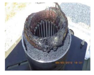
An *inverter-driven compressor* is less likely to fail at start-up because It sees a soft-start, making it MORE RELIABLE
