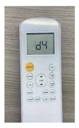
To set Automatic Airflow Adjustment function Select D4 with arrow up button Press Timer on to confirm Wait 10 seconds
