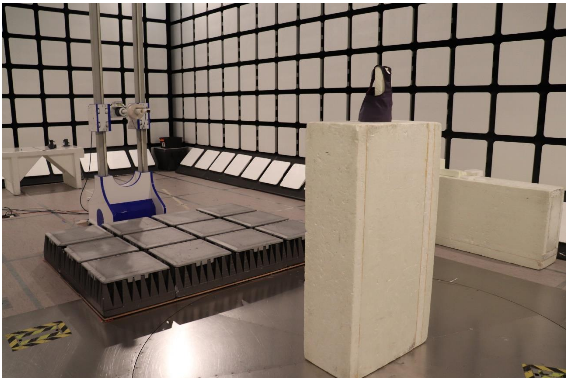
Photograph 6. Test setup for Radiated emissions (18 – 25 GHz)
