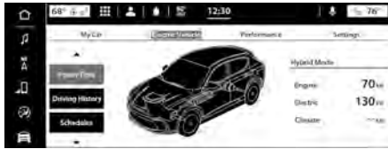
Power Flow Screen
