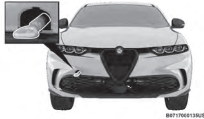
Front Tow Eye Installed
