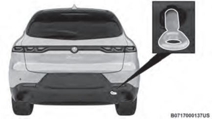
Rear Tow Eye Installed
