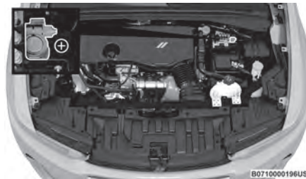
Positive (+) Battery Post
