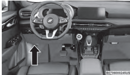
Interior Fuse Box Location
