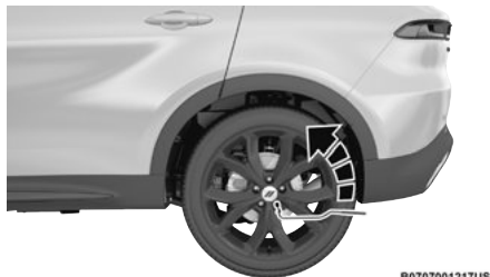
Loosening The Wheel Bolts
