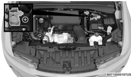
Positive (+) Battery Post
