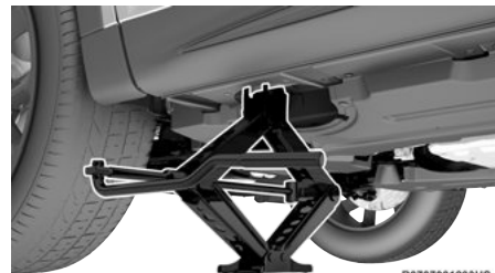
Front Jacking Location
