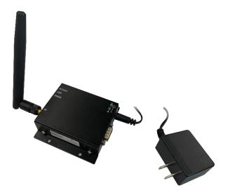
2. Connect the serial cable from the base to your computer; connect the black power adapter (labeled "Base Only") to the base and plug-in.
