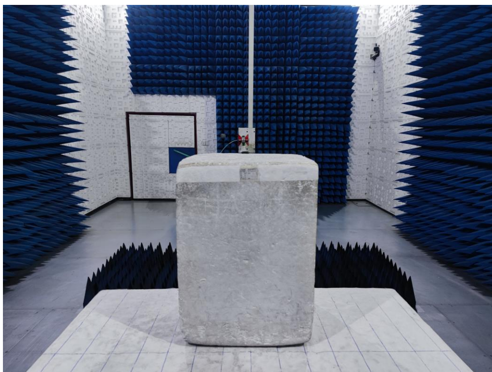
RADIATED EMISSION TEST SETUP ABOVE 1GHz
