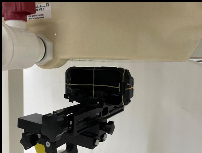
Left Side of EUT with 1.0 cm Gap
