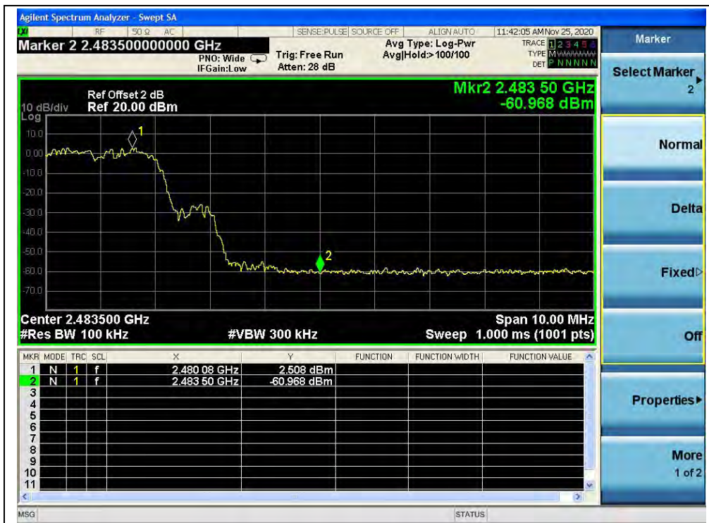
(Band edge with hopping on, Channel 78, 8-DPSK)
