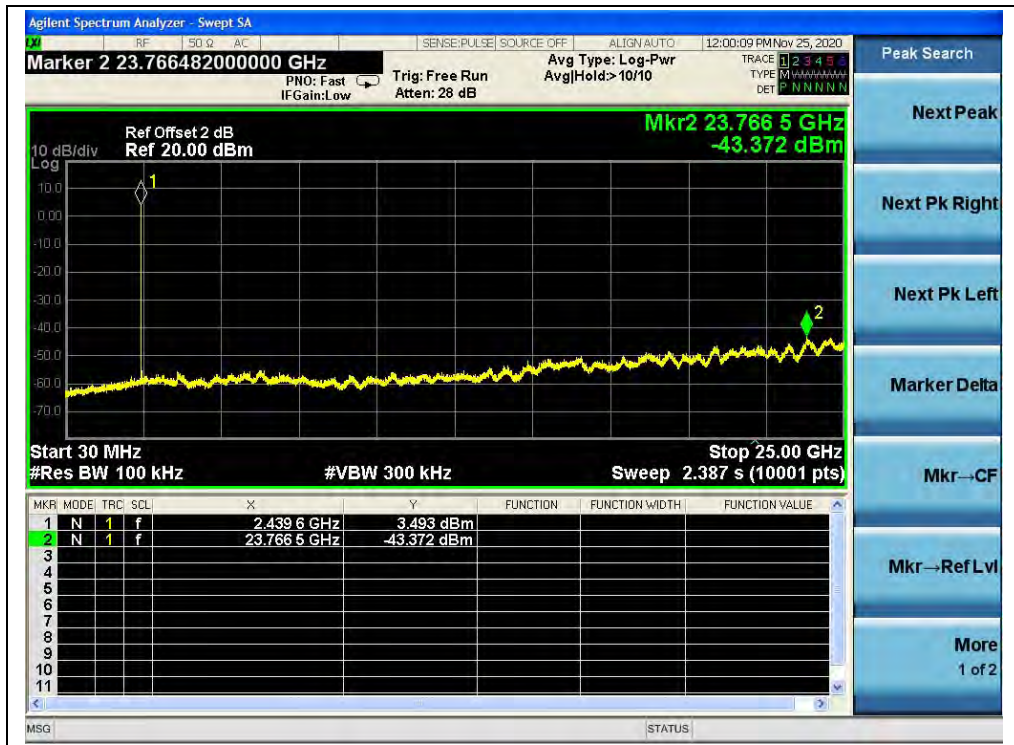
(30MHz to 25GHz, Channel 39, \pi/4 -DQPSK)
