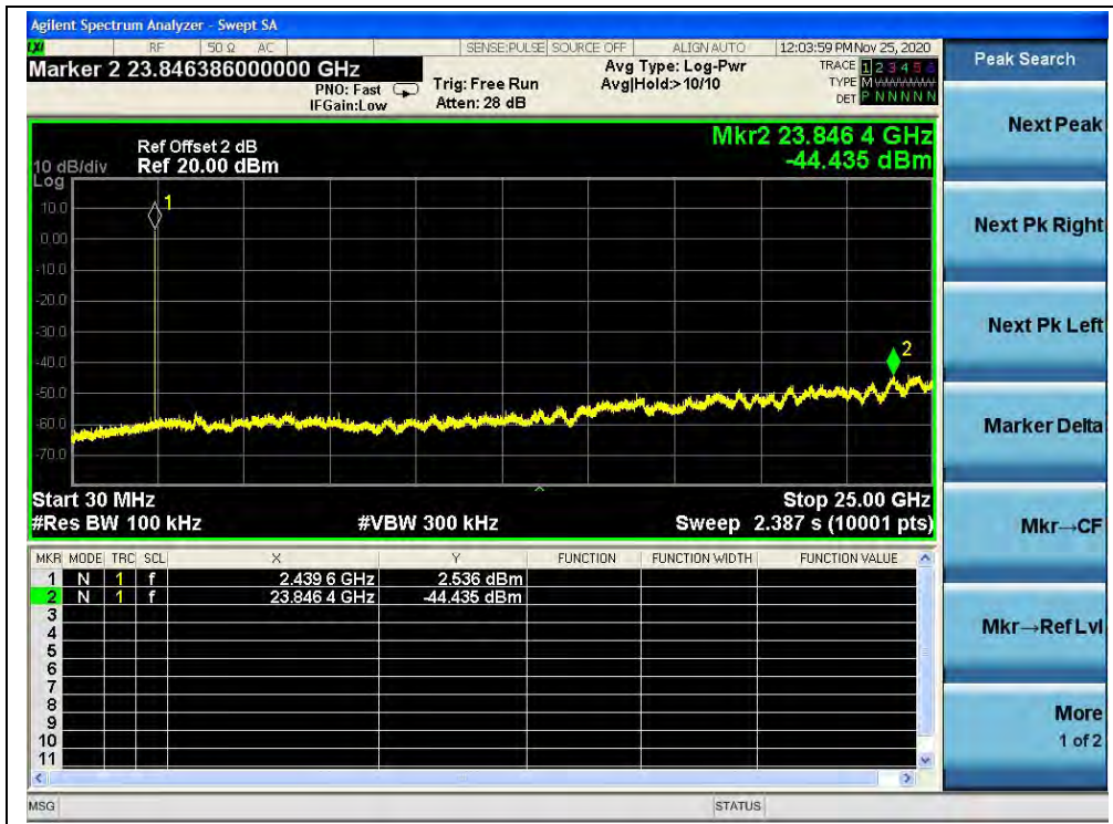
(30MHz to 25GHz, Channel 39, 8-DPSK)
