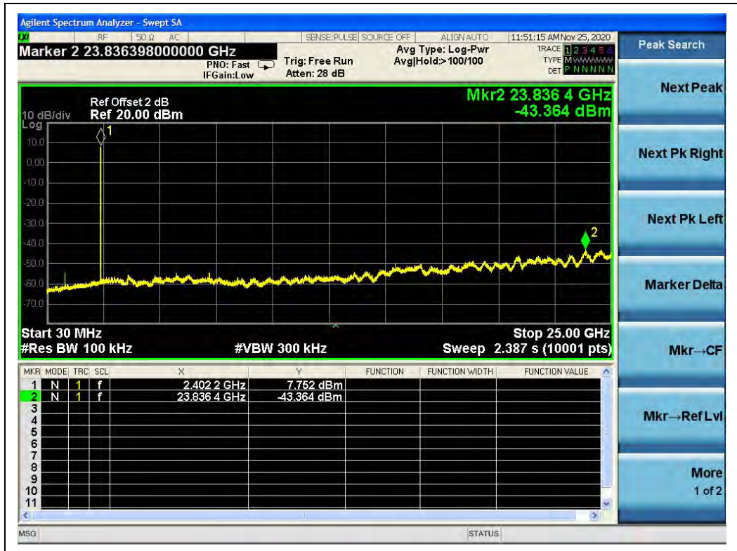
(30MHz to 25GHz, Channel 0, GFSK)
