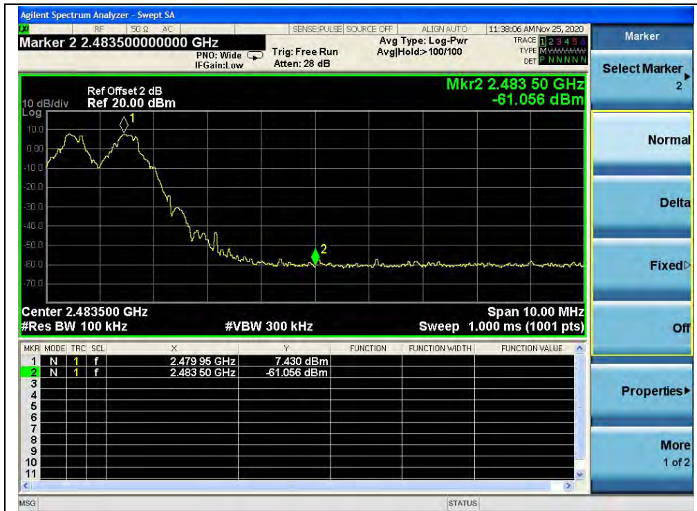
(Band edge with hopping on, Channel 78, GFSK)
