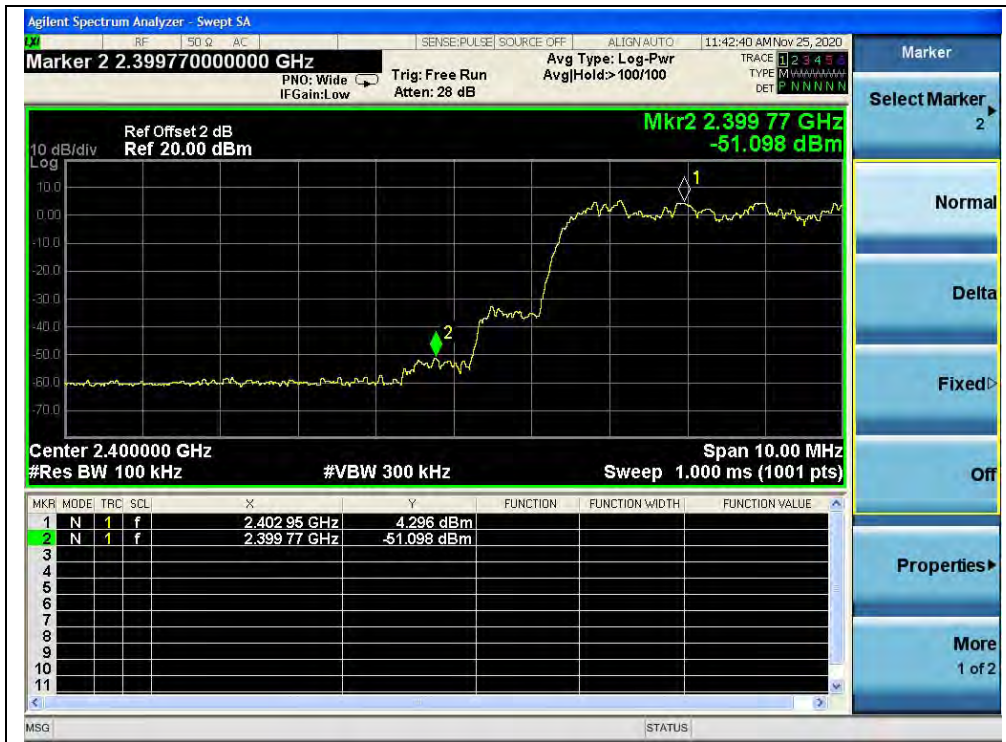
(Band edge with hopping on, Channel 0, 8-DPSK)
