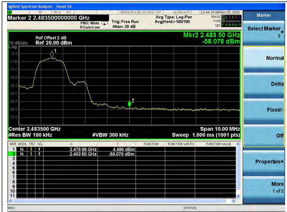
(Band edge, Channel 78, \pi/4 -DQPSK)
