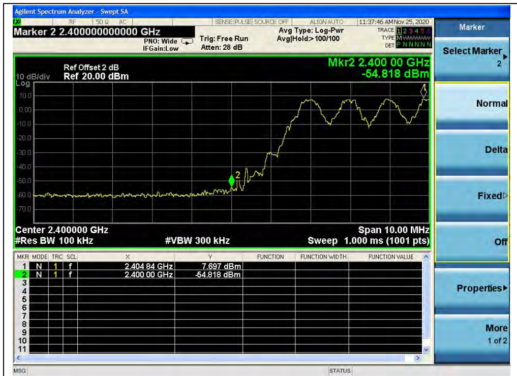
(Band edge with hopping on, Channel 0, GFSK)
