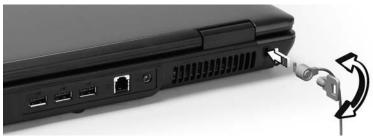
Wrap the computer security lock cable around an immovable object such as a table or handle of a locked drawer. Insert the lock into the notch and turn the key to secure the lock. Some keyless models are also available.
