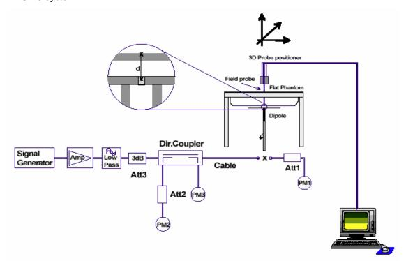
Figure 5-6. System Check Set-up
