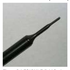
Figure 5-2.ES3DV3 E-field Probe
