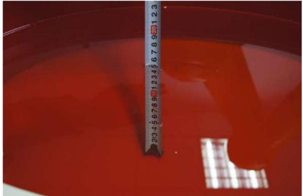
Picture C.3: Liquid depth in the flat Phantom (1900 MHz) (15.3cm deep)
