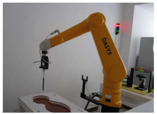
Picture C.1: Specific Absorption Rate Test Layout
