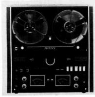
reels. Response 30-25,000 Hz  $\pm 3$  dB; wow & flutter 0.06% at 7½ ips; (S + N)/N 56 dB. Has VU meters, automatic reverse and shutoff, counter, monitoring facilities, solenoid operation.  $18^{1}/16^{\prime\prime}$  H ×  $17^{1}/2^{\prime\prime}$  W ×  $87/6^{\prime\prime}$  D . . . . \$499.95
