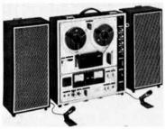
$7^{\prime\prime}$  reels. Response 30-22,000 Hz; wow & flutter 0.09% at 71/2 ips; Built-in electronics with 20 W/ch output. Supplied with speakers and microphones. Has VU meters, automatic shutoff, pause control, echo effects, sound-on-sound, counter, phono input, tone controls, monitoring facilities. Carrying handle included.  $20^{\prime\prime}$  H $\times$   $17^{\prime\prime}$ /8" W $\times$   $11^{\prime\prime}$ /8" D $\dots$ \$449.95
