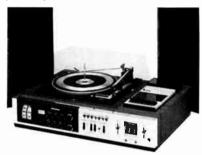
8" woofer & 3" tweeter. Has built-in Phase Q4 matrix to synthesize regular two-channel stereo program material. 20 W/ch dynamic power at 1% HD (121/2 W/ch continuous). Power bandwidth 25-20,000 Hz; response 25-20,000 Hz  $\pm 1 \frac{1}{2}$  dB. FM sensitivity 2.5  $\mu$ V; capture ratio 5.5 dB. Walnut cabinet with dust cover. Comes with pair of microphones. Control center 91/4" × 23½"×15¾"D .....\$399.95
