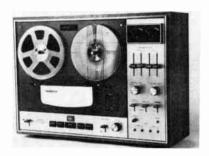
motor stereo unit. Will handle up to 7" reels. Response 40-15,000 Hz  $\pm 2$  dB, wow & flutter less than 0.08% at  $7 \% _2$  ips, (S + N)/N 55 dB. Has VU meters, automatic reverse and shutoff, pause control, echo effects, sound-on-sound, bias adjustment possible, counter, remote-control, monitoring facilities. Dust cover included.  $9 \% _2$ " H  $\times 21 \% _4$ " W  $\times 16 \% _4$ " D . . . . . . . . \$549.95
