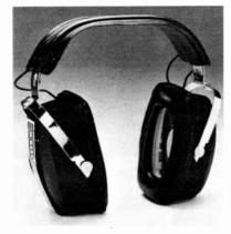
10 mW. Maximum input 2 W; max. output 120 dB. HD 0.6% at 1000 Hz at max. dB. Ambient noise isolation 40 dB at 1000 Hz. 4-8 ohms impedance. Cycolac ear cups and fluid-filled ear cushions. Features patented dual-driver cavity assembly. Comes with 10-ft coiled cord with special strain-relief feature. Black with chrome-plated headband. 18 oz ..... \$45.00
