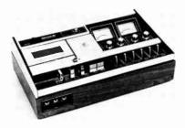
sound-on-sound mixing; Dolby calibration oscillator; tape bias switch for standard and chromium-dioxide tapes; end-of-tape sensing; dual VU meters. Wow & flutter 0.15% (DIN) weighted. Sensitivity: mike 0.65 mV for 0 VU; line 150 mV; Output 1 V; headphone output 0.2 mV at 8 ohms. Response 35-14,000 Hz  $\pm 2$  dB with standard tape. (S+N)/N 50 dB with Dolby off (60 dB at 4000 Hz with Dolby)  $\dots \dots \$  \$299.95
