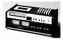
(mixable); two separate erase and record/playback heads. S/(S+N) 51 dB (60 dB with Dolby); wow & flutter 0.07%. Response 30-10,000 Hz with standard tape (30-14,000 Hz with low-noise tape; 30-16,000 Hz with chromium-dioxide tape). Inputs: mike 0.25 mV; line 0.1 V. Output: 0.3 V. Has universal power-line inputs. 7"  $H \times 171/2$ "  $W \times 105/6$ " ..... \$379.50
