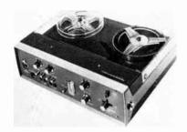
heads. Will handle up to 7" reels. Has automatic level-input controls, mike & line mixing, and built-in speaker. Response 40-16,000 Hz  $\pm 2$  dB at  $71\!\!/_2$  ips, wow 0.1% at  $71\!\!/_2$  ips, (S+N)/N 58 dB unweighted. 13" W  $\times$  10" D  $\times$  4".
