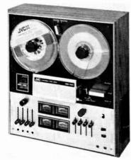
30-20,000 Hz  $\pm 3$  dB at 71/2 ips with low-noise tape. (S + N)/N -53 dB; wow & flutter 0.1% rms at 71/2 ips. 95 kHz bias & erase. Three heads (record, play & erase). Has mike (0.3 mV) & line (80 mV) inputs & line output (0-1 V). Features low-noise or standard tape switch. 161/6° × 175/6° H × 73/6° D . . . . . . . . . . \$449.95
