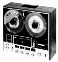
18,000 Hz  $\pm 3$  dB at 71/2 ips with low-noise tape. (S+N)/N-52 dB; wow & flutter 0.1% at 71/2 ips. 57 kHz bias & erase. Has two heads (record/play & erase), mike (0.5 mV) & line (80 mV) inputs, and line output (0-1.2 V). Features low-noise or standard tape switch.  $71/6 \text{ mV} \times 131/2 \text{ m} \times 131$
