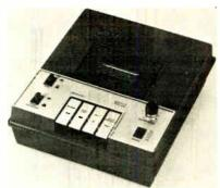
um-dioxide tape (regular equalization also provided). Response 30-15,000 Hz  $\pm 2$  dB; wow & flutter less than 0.2% DIN. Has hysteresis synchronous motor, automatic shut-off, digital counter. Overall size 3%e'' H  $\times$  9%e'' W  $\times$  10%e'' D
