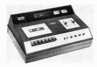
panded-scale VU meters; independent record-level controls; auto-stop; counter on mike inputs. Response 30-12,000 Hz (CrO $_2$  14,000 Hz); (S + N)/N 50 dB. Wow & flutter (weighted) 0.2% rms. Sensitivity: mike 0.2 mV (±3 dB) 0 VU at 1500 ohms; aux. 100 mV (±2 dB) for 0 VU at 5000 ohms. Output 1 volt (±2 dB) for 0 VU at 5000 ohms.  $5\frac{1}{2}$ " ×  $15\frac{1}{2}$ " ×  $10\frac{1}{2}$ " D . . . \$249.95
