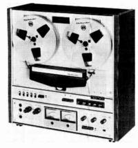
mV) & line (80 mV) inputs. Output 0.775 V. Features bidirectional recording and automatic repeat playback. Six heads (2 each erase, record, playback). Has 3 motors. Tape bias switch for standard or low-noise tapes. Features sound-on-sound, sound-with-sound, echo, and tape monitoring. 16% × 17% × 6% ° 0.\$579.95
