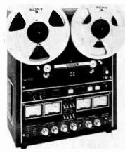
channel. Features vari-speed pitch control and Sony's "Synchro Trak" for precise synchronization of each track. Response 30-18,000 Hz  $\pm 2$  dB at  $7V_2$  ips (S + N)/N 56 dB with standard tape (59 dB with SLH-180 tape). Wow & flutter 0.04% at  $7V_2$  ips. Has four VU meters, sound-on-sound capabilities, record equalization switch for standard or low-noise, high-output tape. 17%"  $\times$  22"  $\times$  10" D. . . . . . . . . . . . \$1795.00
