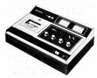
tra-longlife heads. Wow & flutter 0.2% (S + N) /N 55 dB (with Dolby), 45 dB (without). Response 20-13,000 Hz (standard tape), 20-14,000 Hz (chromium-dioxide). Has two VU meters, memory rewind, lockable pause control, automatic stop, mike/line selector, electronically controlled motor speed.  $15\%s'' \times 10\%s'' \times 5''$ . ... \$249.95
