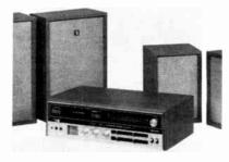
4-channel playback; and four separately housed speaker systems. Two front speakers  $12''\times171/2''\times71/4''$ ; two rear speakers  $81/4''\times12''\times71/4''$  D. Front speakers are 2-way designs, each with 61/2'' & 21/2'' speakers; rear speakers have 61/2'' units. Tape deck response 50-12,000 Hz. (S+N)/N 50 dB; wow & flutter 0.25%. 161/4 W/ch (65 W total) dynamic power at 5% HD. Has SQ matrix decoder and separate record/playback amp.  $20''\times6''\times121/2''$  . \$329.95
