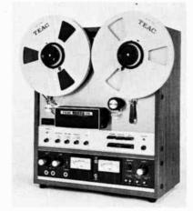
playback). Two speeds  $(3\frac{3}{4} \& 7\frac{1}{2} \text{ ips})$ , 3 motors. Will handle 7" &  $10\frac{1}{2}$ " reels. Response 30-20,-000 Hz  $\pm 3$  dB at  $7\frac{1}{2}$  ips. (S+N)/N-58 dB; HD 1% at 1000 Hz at normal listening levels. Has mike (0.25 mV) and line (0.1 V) inputs. Line output 0.3 V,  $2\frac{1}{6}$ "  $\times 17\frac{5}{6}$ " W  $\times 9\frac{1}{2}$ " D , \$999.50
