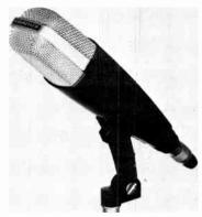
$\mu$ bar ±3 dB at 1 kHz. EIA rating -145.8 dB. Output level -53 dBm (1 mW/10 dynes/cm²). Has front-to-back ratio 18 dB, -2 dB and a variable bass attenuator. Fitted with XLR connector. 14 ounces.  $7" \times 17'6" \times 11^3/16" \dots \$134.00$
