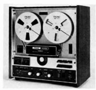
heads (6 head functions). Will handle up to 7" reel. Response 30-20,000 Hz  $\pm 3$  dB, wow & flutter 0.05% at 7½ ips, (S+N)/N 58 dB. Has braking, VU meters, automatic reverse and shutoff, pause control, bias adjustment, counter, separate bias & equalizer switches and monitoring facilities. Remote control available optional extra. 17% "H  $\times$  18" W  $\times$  9% 16" D . \$599.50
