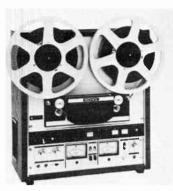
flutter 0.03% at  $7\frac{1}{2}$  ips; (S+N)N 57 dB. Has VU meters, automatic shutoff, pause control, echo effects, sound-on-sound, bias adjust, counter, solenoid operation, monitoring facilities. Remote control optional extra.  $19^{3}\frac{1}{4}$ " H  $\times 17^{1}\frac{1}{2}$ " W  $\times 10^{11}$  D................\$895.00 Model 850-2. Same as Model 850-4 except two-track ................\$895.00
