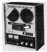
rite heads. Response 30-22,000 Hz at 71/2 ips, wow & flutter less than 0.1% at 71/2 ips, (S+N)/N better than 50 dB. Has VU meters, automatic shutoff, pause control, sound-on sound, counter, remote control (optional extra), solenoid operation, and monitoring. 20"  $H \times 17$ " W×71/8" D..... Model RS-715US. Similar to RS-714US except this model includes an automatic reverse fea-
