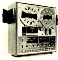
reel tape speeds  $17_8$ ,  $37_4$  &  $77_2$  ips; wow & flutter 0.12% rms at  $77_2$  ips. Response 30-22,000 Hz  $\pm 3$  dB at  $77_2$  ips. Has four mike (0.8 mV) & line (80 mV) inputs. Universal power supply.  $167_6$ ° ×  $177_6$ ° ×  $99_6$ ° D . . . . . . . \$499.95
