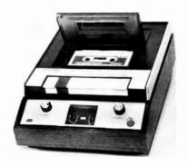
and auxiliary inputs, and preamp outputs. Response 50-10,000 Hz ±3 dB (playback-only response 40-12,000 Hz ±2 dB). Wow & flutter 0.25% rms. Oiled-walnut case. 105/8" × 71/4" × ..... \$99.95
