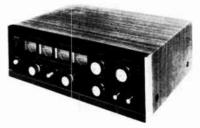
tion and system control, including four VU meters but without any power amplifiers
