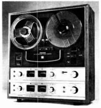
channel stereo. One motor drive with automatic reverse. Two speeds ( $7^{1/2}$ ,  $3^{3/4}$  ips), wow & flutter 0.12% at  $7^{1/2}$  ips. Response 50-15,000 Hz  $\pm 2$  dB  $7^{1/2}$  ips, (S + N)/N 55 dB. Has mike (0.3 mV) and line (30 mV) inputs. Output 0.775 V at 50,000 ohms.  $17^{\text{m}}$  W  $\times$   $18^{3/8}$  H  $\times$   $8^{3/8}$  ...... \$599.95
