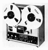
$7\frac{1}{2}$  ips, wow & flutter 0.06% at  $7\frac{1}{2}$  ips, (S + N)/ N 58 dB. Has mike (0.25 mV) and two line inputs (0.1 V & 0.3 V), 3 heads (erase, record & play). Will handle up to  $10\frac{1}{2}$  reels. Features three motors (1 dual-speed hysteresis sync capstan motor and 2 eddy-current induction reel motors); VU meters; automatic shutoff; bias adjust; and monitoring facilities.  $15\frac{1}{2}$  "  $\times 9\frac{1}{2}$   $\times 9\frac{1}{2}$
