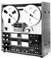
mal level. Has inputs for mike (0.25 mV) and line (0.1 V) and line output (0.3 V). Features "Simul-Sync" for each head permitting synchronization of any of the remaining three tracks; 3-motor transport; dual bias-level switch for conventional & high performance tapes; mike/line mixing; separate record & playback amp; four VU meters.  $18^3/4$ " ×  $17^9/8$ " ×  $8^9/4$ " D. . . . . . . . . . . \$759.50
