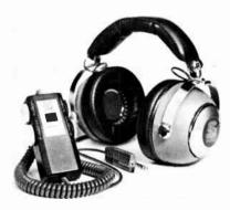
Dynamic design with remote control for volume & tone, 13-ft coiled cord. Response 40-11,000 Hz  $\pm 3$  dB. Sensitivity 100 dB SPL (at 0.11-V at 1000 Hz). Max. input 0.5 W rms; dist. 1.0% with 115 dB SPL. Input 12 ohms imp. Features two-way design with separate woofer & tweeter with LC crossover network. 28 ounces .... \$74.95 Model 5741. Same as used on Dynaphase Seventy-Five. Separate volume & tone controls
