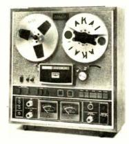
heads. Will handle up to 7" reels. Response 30-24,000 Hz  $\pm 3$  dB, wow & flutter 0.08%, (S + N)/N 50 dB, all at  $7\frac{1}{2}$  ips. Has VU meters, counter, and remote control (optional extra). Features automatic reverse and shutoff, pause control, and sound-on-sound facilities.  $17^{"} \times 18^{"} \text{ W} \times 10^{"} \text{ D}$  \$499.95
