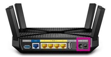
**4.** You can connect devices such as PC desktops, laptops or gaming consoles by plugging Ethernet cables from the device to any of the four **yellow Ethernet ports**, or you can connect devices via WiFi.
