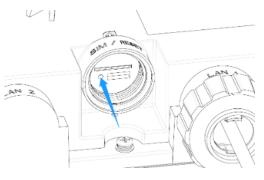
**Note:** During the Reset process, make sure the power adaptor is connected to the device to ensure an uninterrupted power supply.
