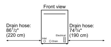
The electrical junction box and water inlet are at the front of the appliance, the drain at the rear.
