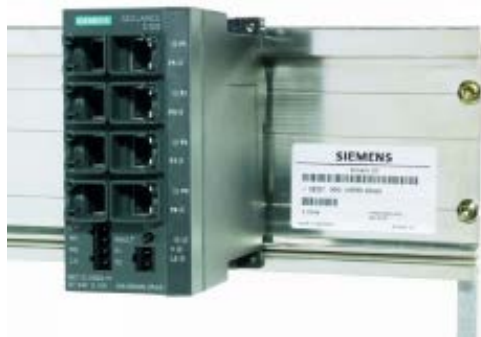
Figure 4-3 Installation on a SIMATIC S7-300 standard rail
