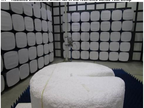
1.2 Radiated Spurious Emissions Test Setup
