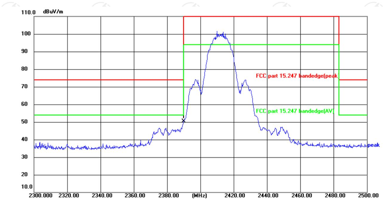
Site: #3 3m Anechoic Chamber      Polarization: **Horizontal**      Temperature: 22.8(°C)      Humidity: 54 %
