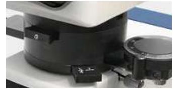
Bertrand lens, \lambda Slip, 360° rotatable analyser (removable)
