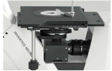
Specimen stage and illumination unit
