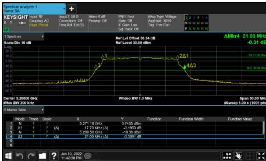
Figure 290 - Core 1 (B) 5280 MHz (CH56) 26 dB and 99% Bandwidth
