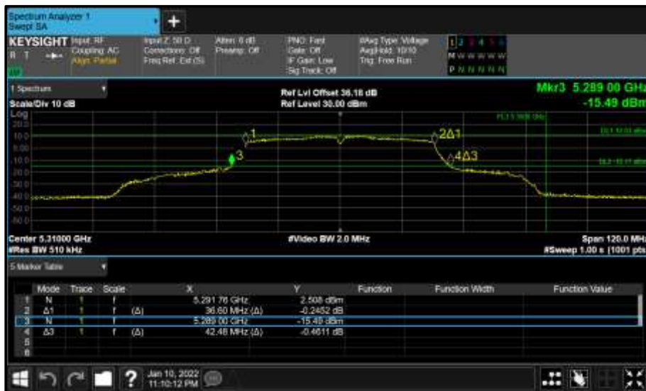
Figure 300 - Core 0 (A) 5310 MHz (CH62) 26 dB and 99% Bandwidth
