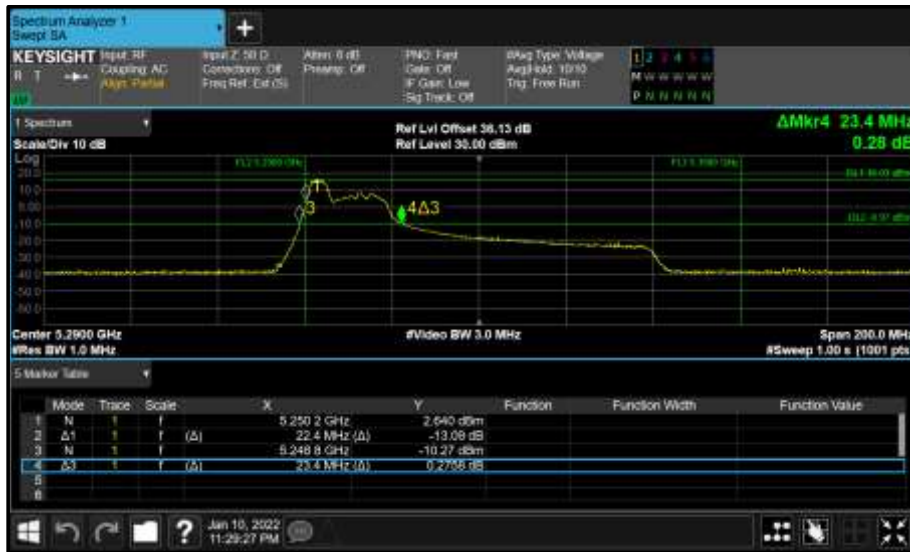
Figure 369 - Core 0 (A) 5290 MHz (CH58) 26 dB and 99% Bandwidth
