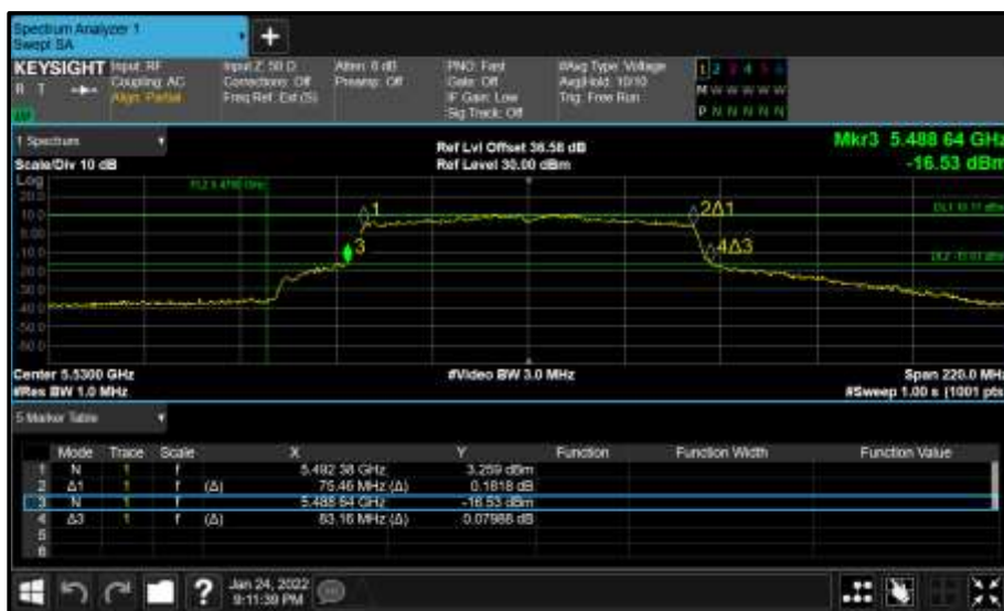
Figure 433 - Core 1 (B) 5530 MHz (CH106) 26 dB and 99% Bandwidth
