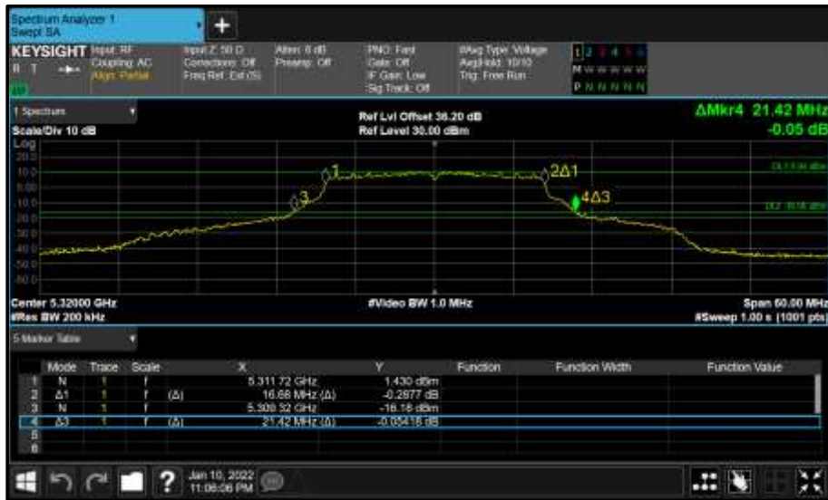
Figure 283 - Core 0 (A) 5320 MHz (CH64) 26 dB and 99% Bandwidth
