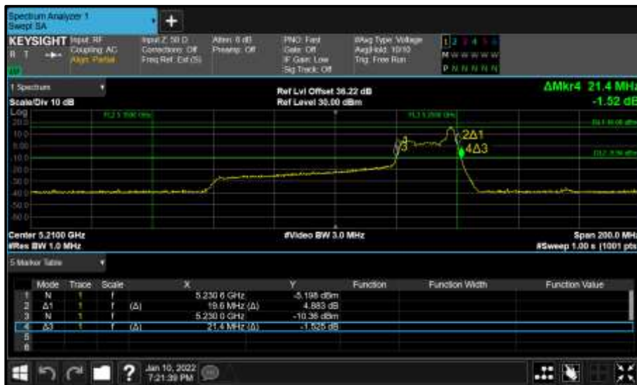
Figure 268 - Core 1 (B) 5210 MHz (CH42) 26 dB and 99% Bandwidth
