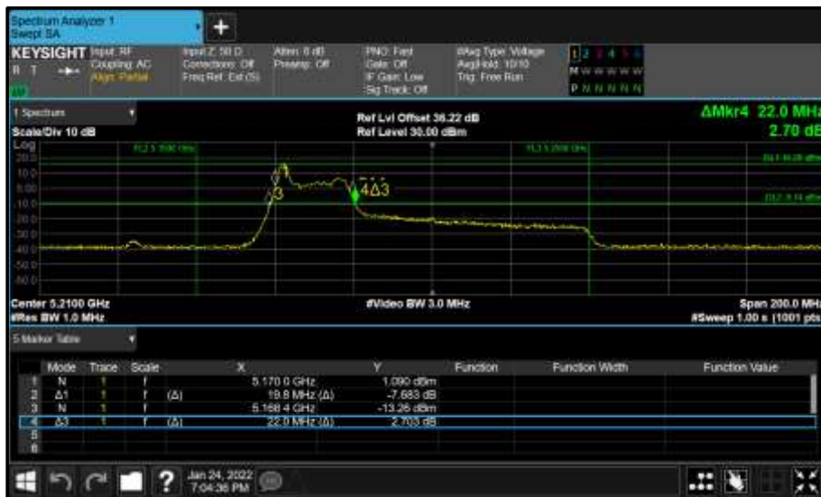
Figure 274 - Core 1 (B) 5210 MHz (CH42) 26 dB and 99% Bandwidth
