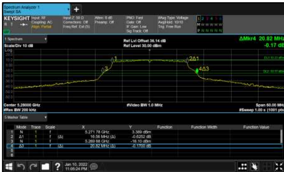
Figure 282 - Core 0 (A) 5280 MHz (CH56) 26 dB and 99% Bandwidth
