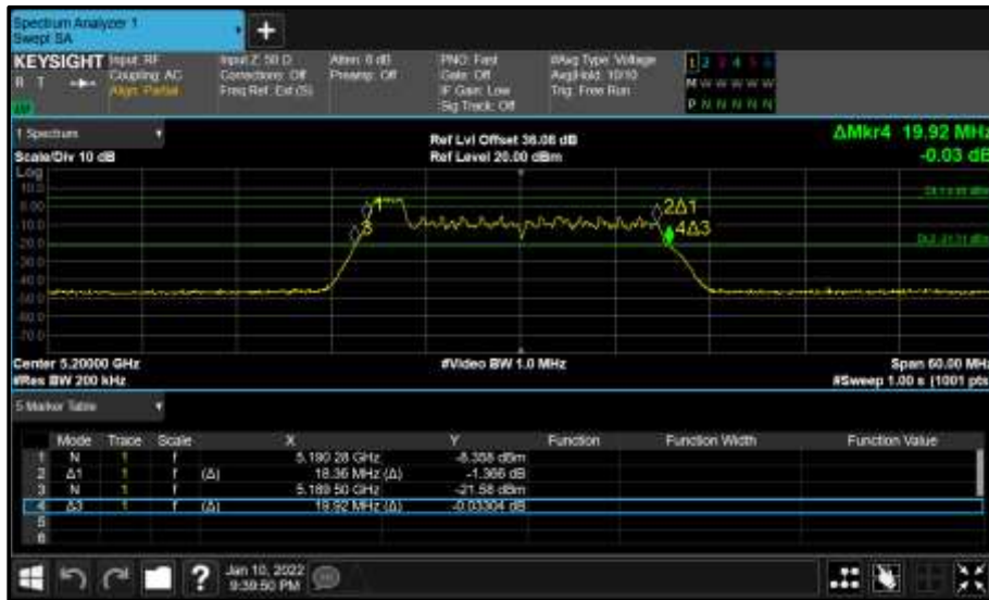
Figure 195 - Core 0 (A) 5200 MHz (CH40) 26 dB and 99% Bandwidth
