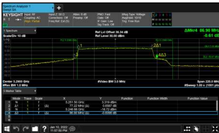
Figure 366 - Core 1 (B) 5290 MHz (CH58) 26 dB and 99% Bandwidth
