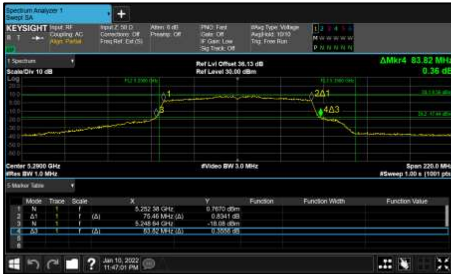
Figure 310 - Core 0 (A) 5290 MHz (CH58) 26 dB and 99% Bandwidth
