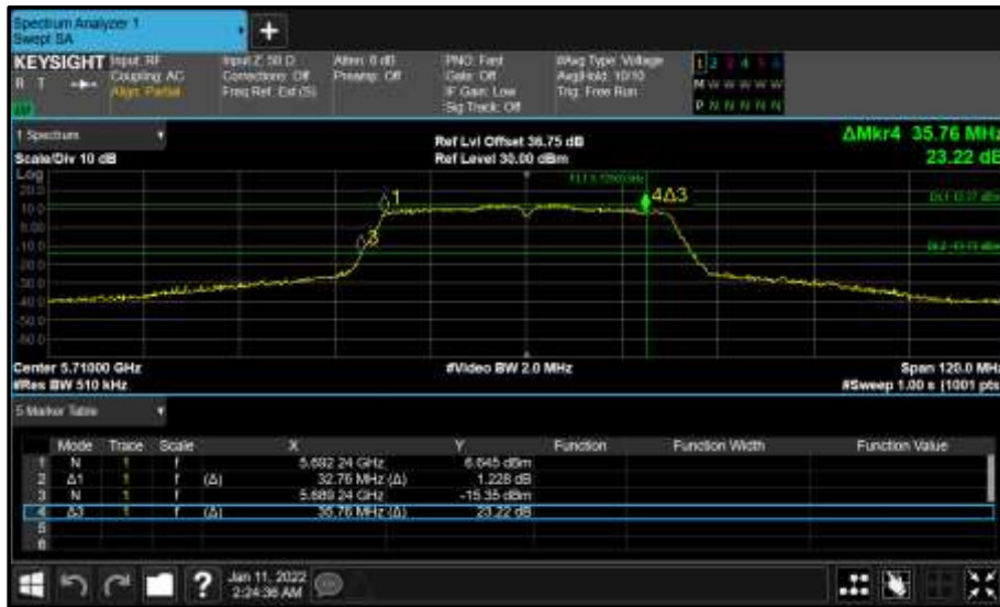
Figure 413 - Core 0 (A) 5710 MHz (CH142) 26 dB and 99% Bandwidth
