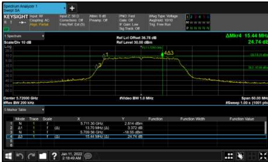
Figure 393 - Core 0 (A) 5720 MHz (CH144) 26 dB and 99% Bandwidth
