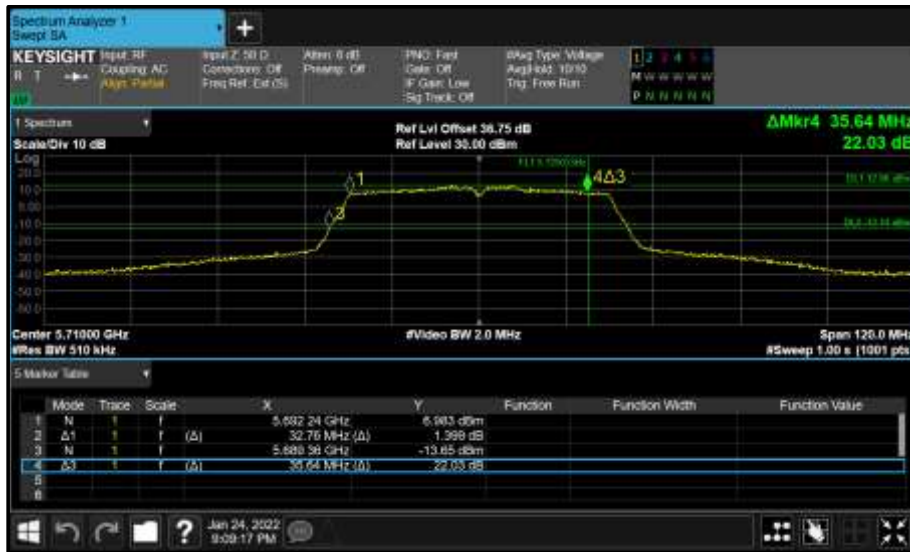
Figure 421 - Core 0 (A) 5710 MHz (CH142) 26 dB and 99% Bandwidth
