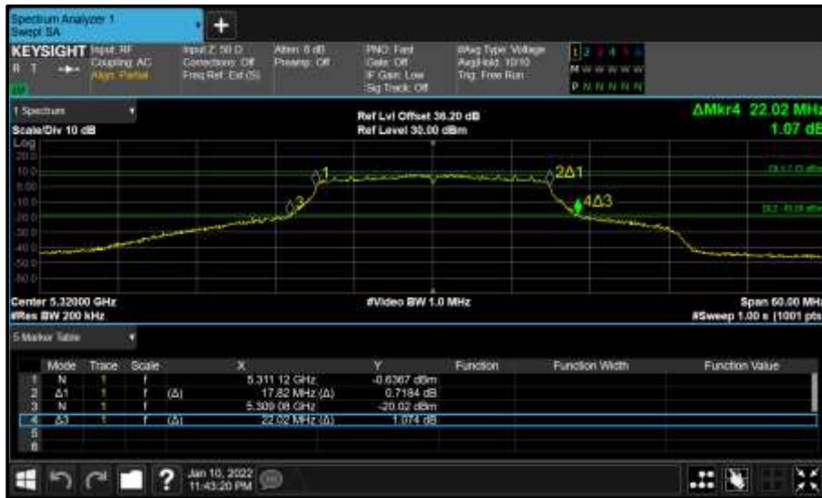
Figure 291 - Core 0 (A) 5320 MHz (CH64) 26 dB and 99% Bandwidth
