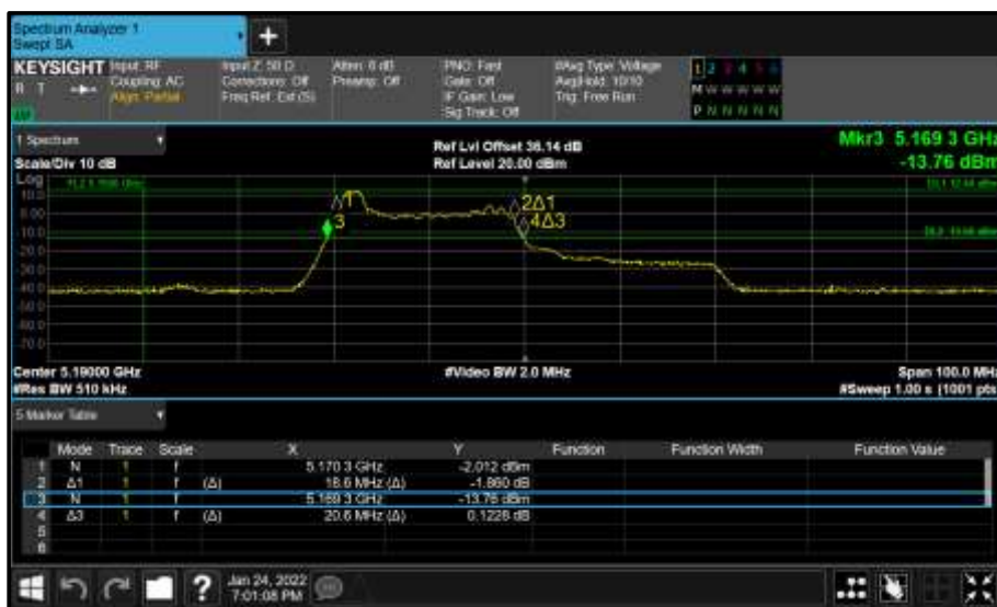
Figure 244 - Core 1 (B) 5190 MHz (CH38) 26 dB and 99% Bandwidth
