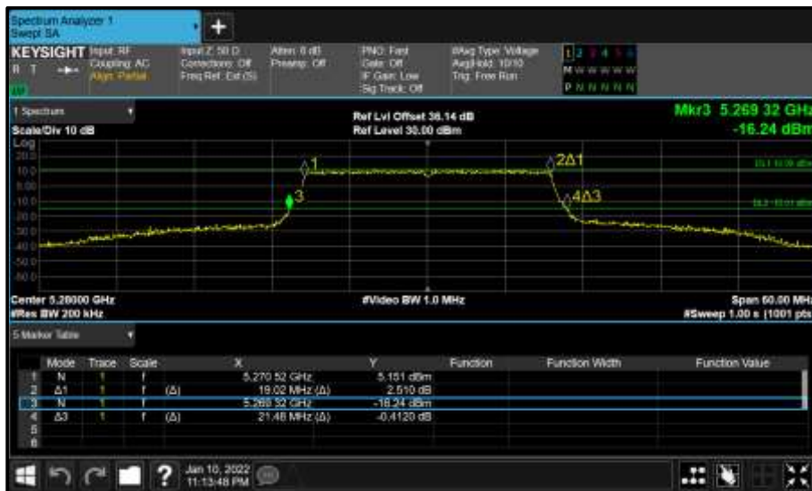
Figure 315 - Core 0 (A) 5280 MHz (CH56) 26 dB and 99% Bandwidth
