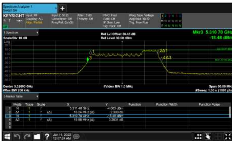
Figure 337 - Core 1 (B) 5320 MHz (CH64) 26 dB and 99% Bandwidth
