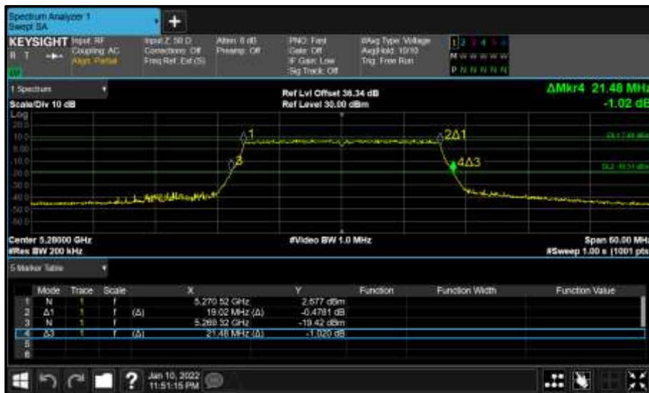
Figure 320 - Core 1 (B) 5280 MHz (CH56) 26 dB and 99% Bandwidth
