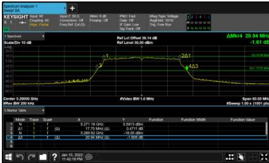
Figure 289 - Core 0 (A) 5280 MHz (CH56) 26 dB and 99% Bandwidth
