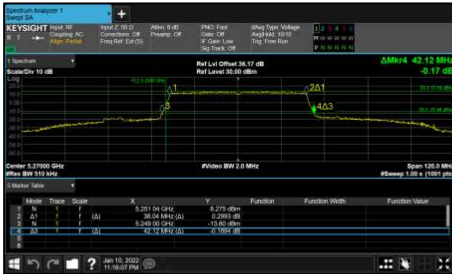
Figure 344 - Core 0 (A) 5270 MHz (CH54) 26 dB and 99% Bandwidth
