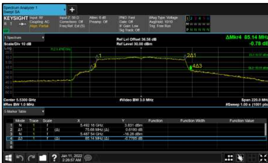
Figure 427 - Core 1 (B) 5530 MHz (CH106) 26 dB and 99% Bandwidth
