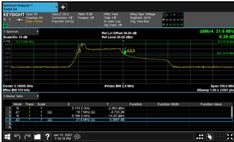
Figure 235 - Core 0 (A) 5190 MHz (CH38) 26 dB and 99% Bandwidth
