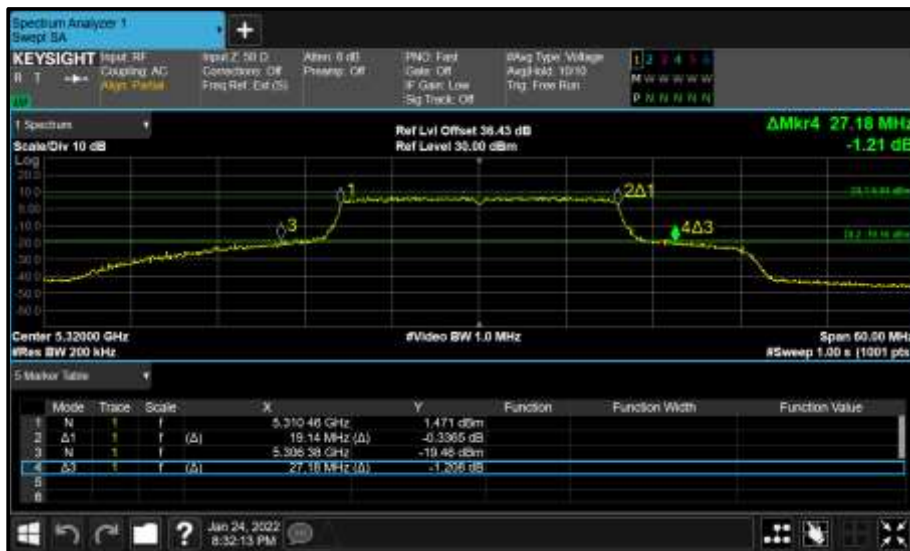
Figure 328 - Core 1 (B) 5320 MHz (CH64) 26 dB and 99% Bandwidth
