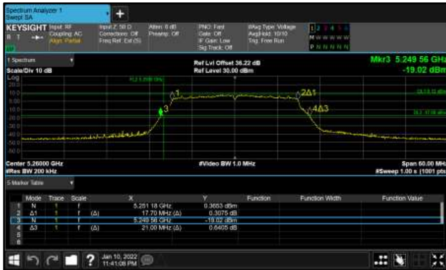
Figure 287 - Core 0 (A) 5260 MHz (CH52) 26 dB and 99% Bandwidth
