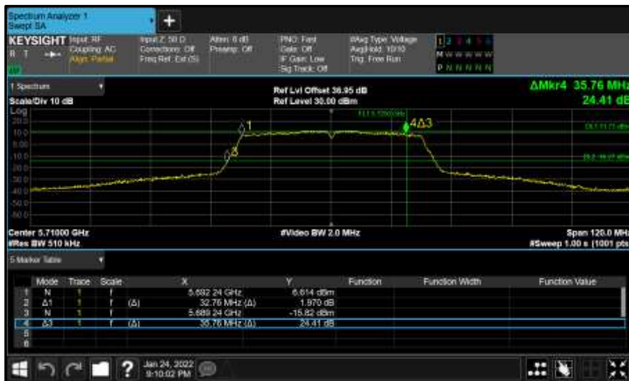
Figure 422 - Core 1 (B) 5710 MHz (CH142) 26 dB and 99% Bandwidth
