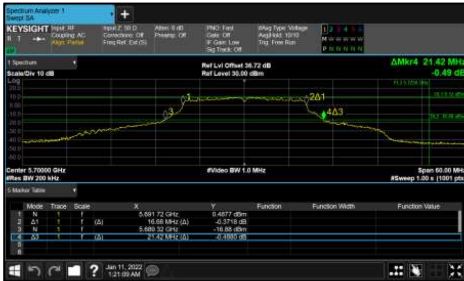
Figure 381 - Core 0 (A) 5700 MHz (CH140) 26 dB and 99% Bandwidth
