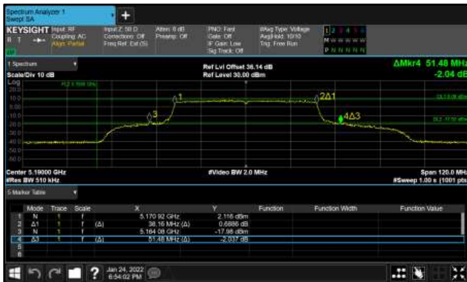
Figure 224 - Core 1 (B) 5190 MHz (CH38) 26 dB and 99% Bandwidth
