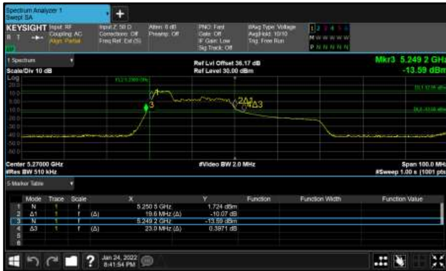
Figure 360 - Core 0 (A) 5270 MHz (CH54) 26 dB and 99% Bandwidth
