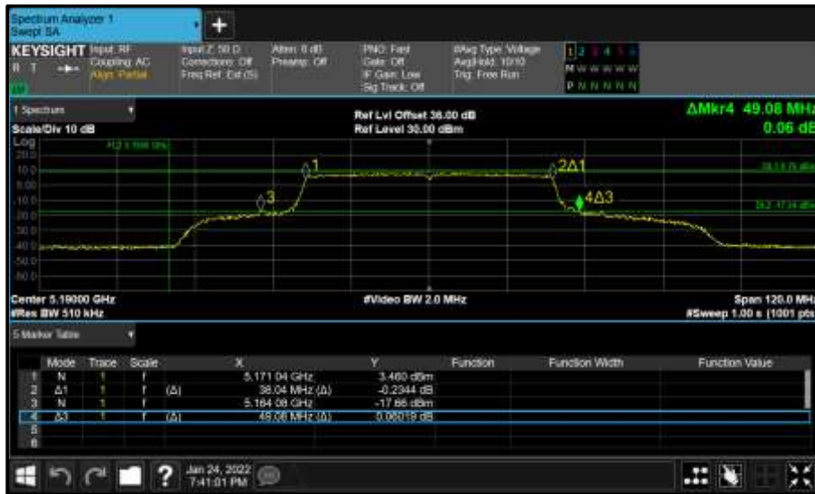
Figure 227 - Core 0 (A) 5190 MHz (CH38) 26 dB and 99% Bandwidth
