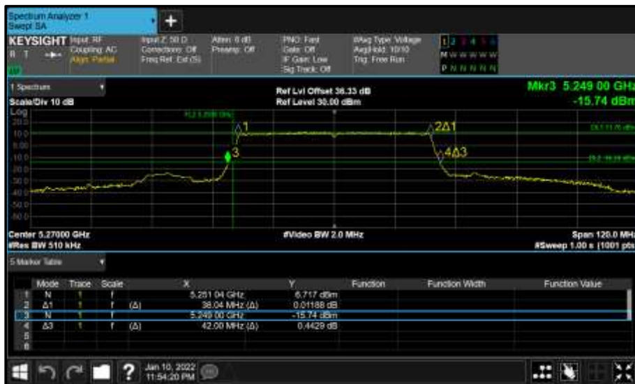
Figure 347 - Core 1 (B) 5270 MHz (CH54) 26 dB and 99% Bandwidth
