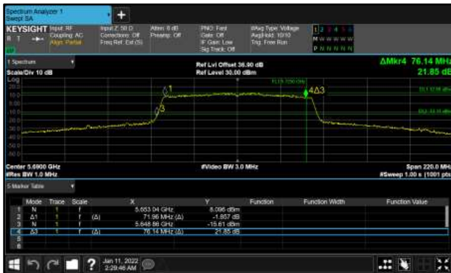
Figure 431 - Core 1 (B) 5690 MHz (CH138) 26 dB and 99% Bandwidth
