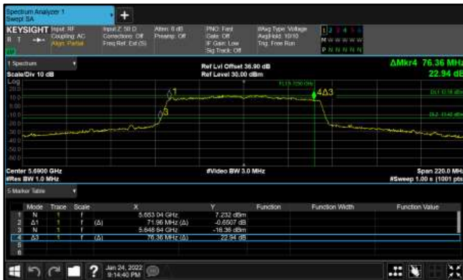
Figure 437 - Core 1 (B) 5690 MHz (CH138) 26 dB and 99% Bandwidth
