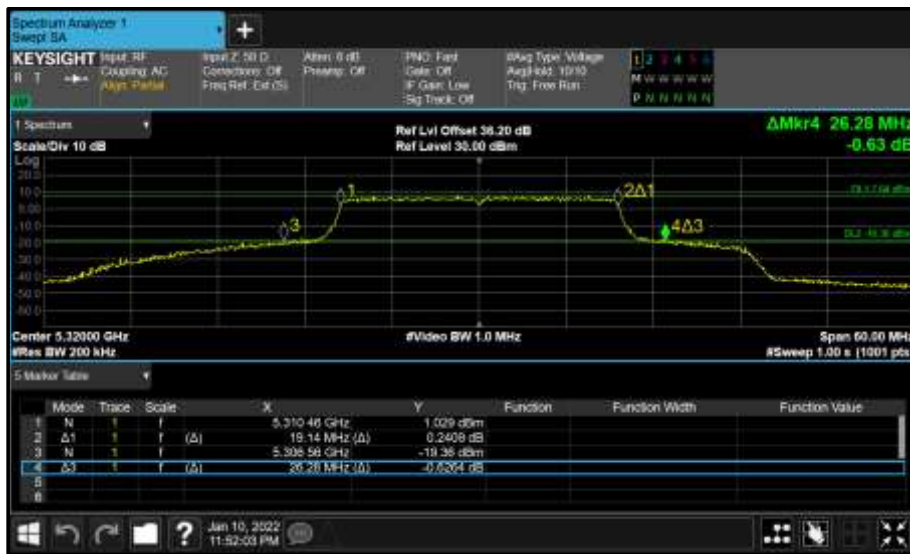
Figure 321 - Core 0 (A) 5320 MHz (CH64) 26 dB and 99% Bandwidth
