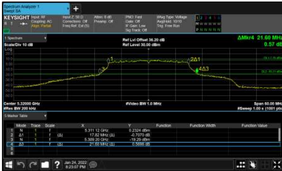
Figure 297 - Core 0 (A) 5320 MHz (CH64) 26 dB and 99% Bandwidth
