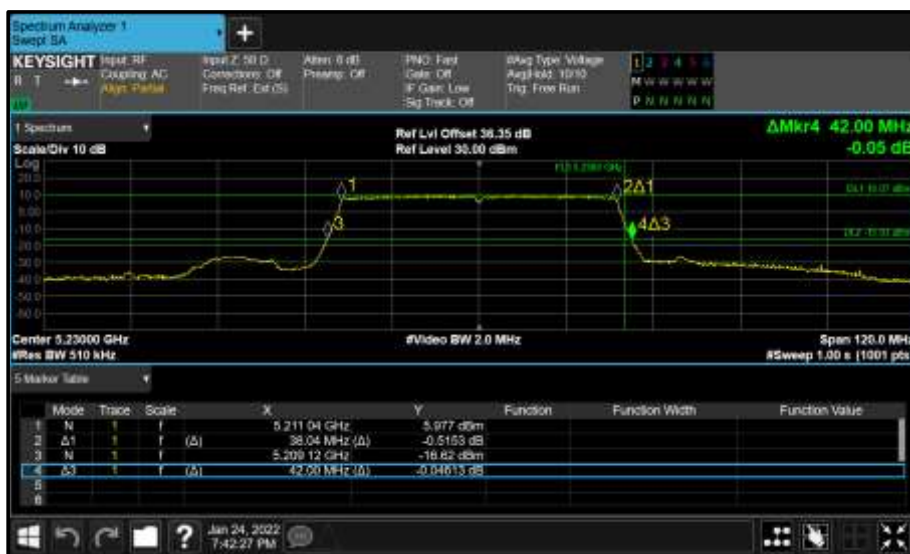
Figure 230 - Core 1 (B) 5230 MHz (CH46) 26 dB and 99% Bandwidth
