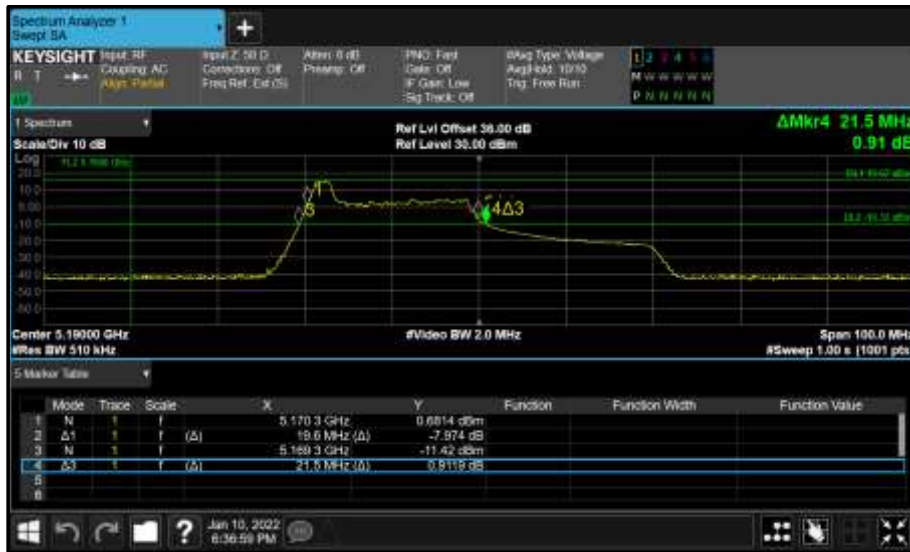
Figure 231 - Core 0 (A) 5190 MHz (CH38) 26 dB and 99% Bandwidth
