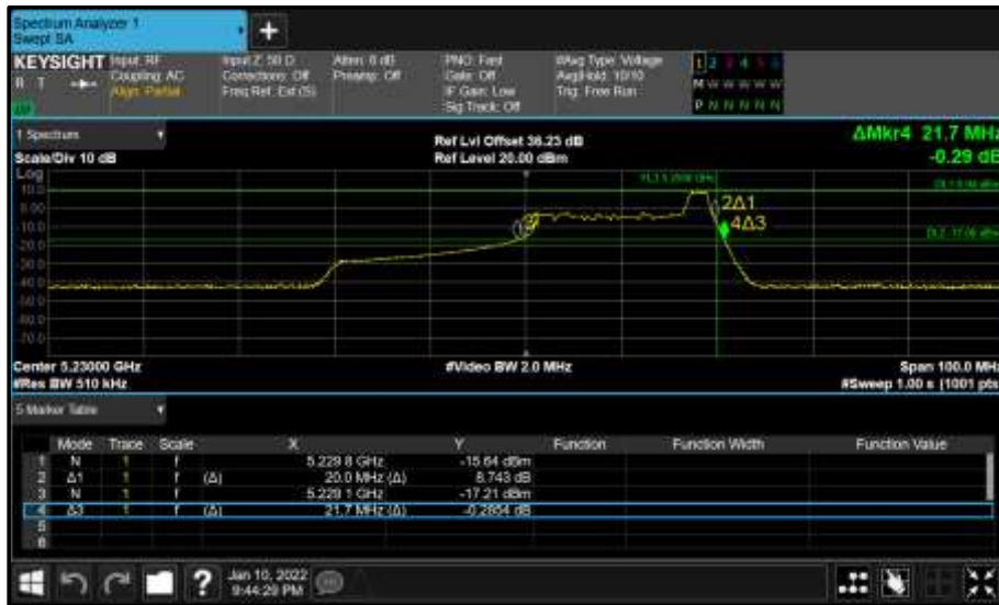
Figure 241 - Core 0 (A) 5230 MHz (CH46) 26 dB and 99% Bandwidth
