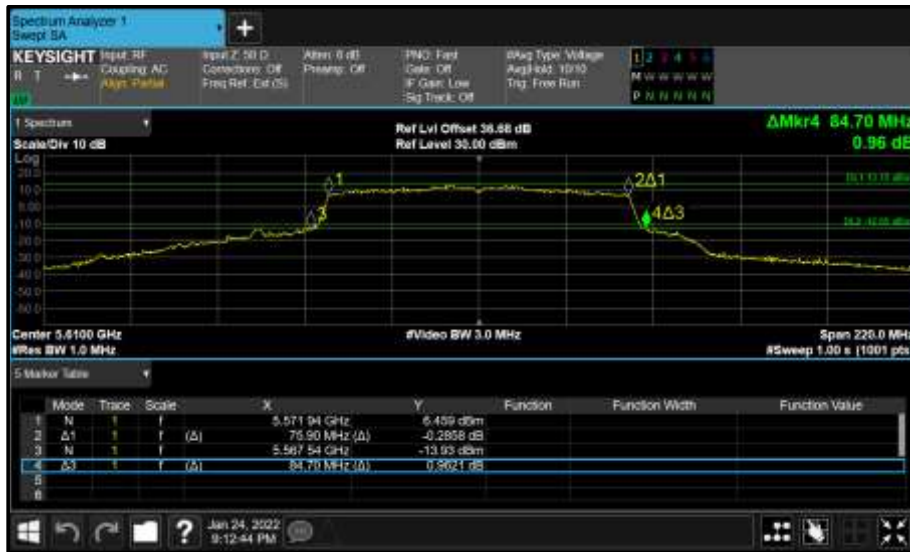
Figure 434 - Core 0 (A) 5610 MHz (CH122) 26 dB and 99% Bandwidth
