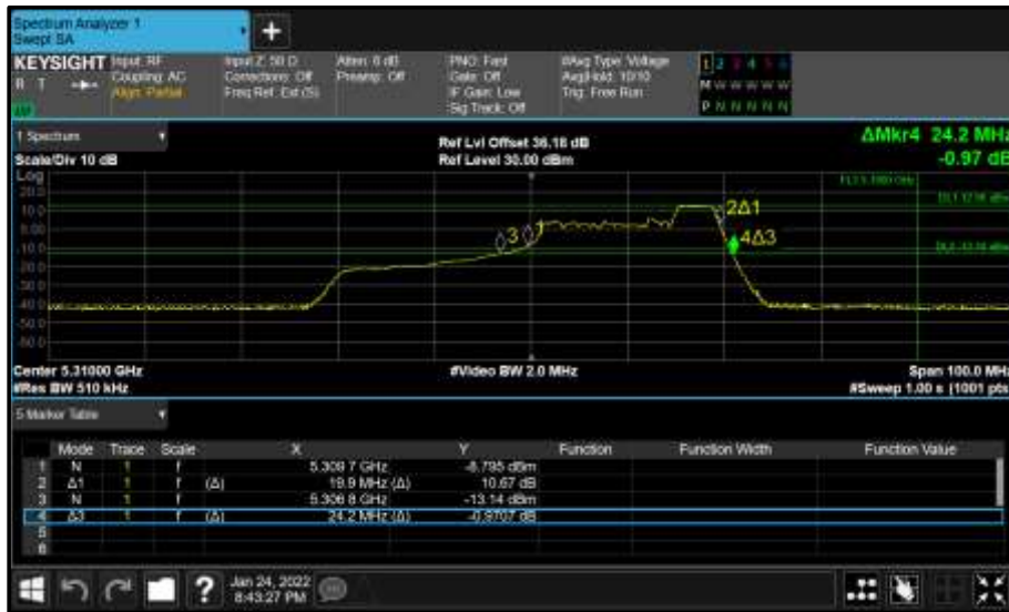
Figure 362 - Core 0 (A) 5310 MHz (CH62) 26 dB and 99% Bandwidth
