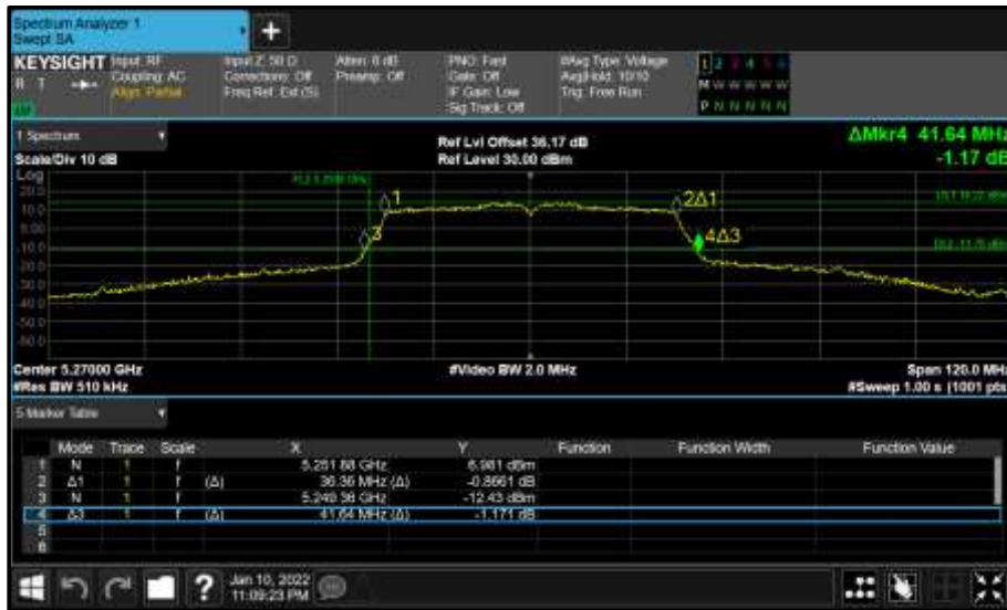
Figure 299 - Core 0 (A) 5270 MHz (CH54) 26 dB and 99% Bandwidth
