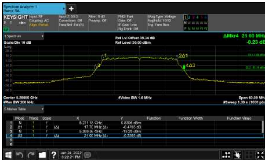
Figure 296 - Core 1 (B) 5280 MHz (CH56) 26 dB and 99% Bandwidth
