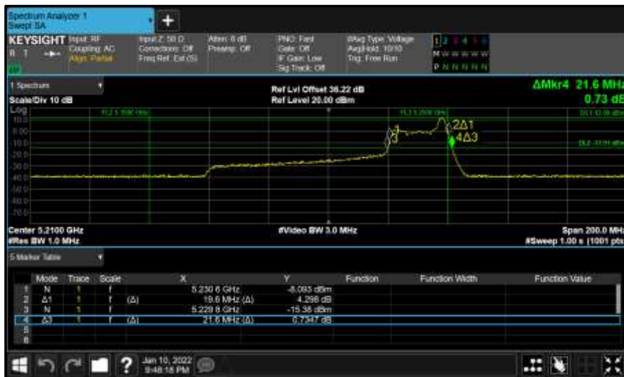
Figure 272 - Core 1 (B) 5210 MHz (CH42) 26 dB and 99% Bandwidth
