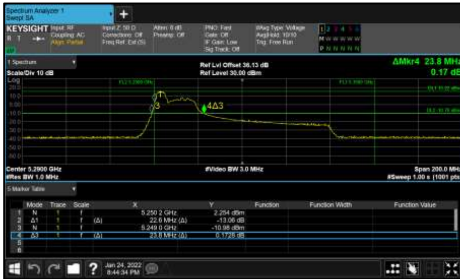
Figure 375 - Core 0 (A) 5290 MHz (CH58) 26 dB and 99% Bandwidth
