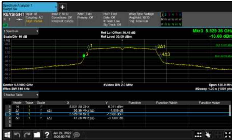
Figure 417 - Core 0 (A) 5550 MHz (CH110) 26 dB and 99% Bandwidth
