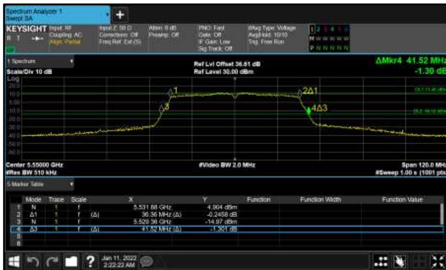
Figure 410 - Core 1 (B) 5550 MHz (CH110) 26 dB and 99% Bandwidth
