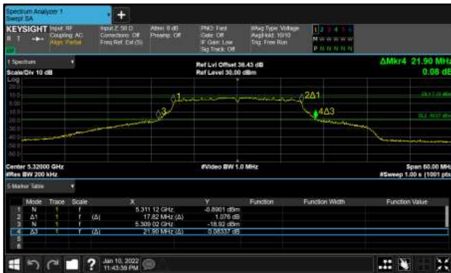
Figure 292 - Core 1 (B) 5320 MHz (CH64) 26 dB and 99% Bandwidth
