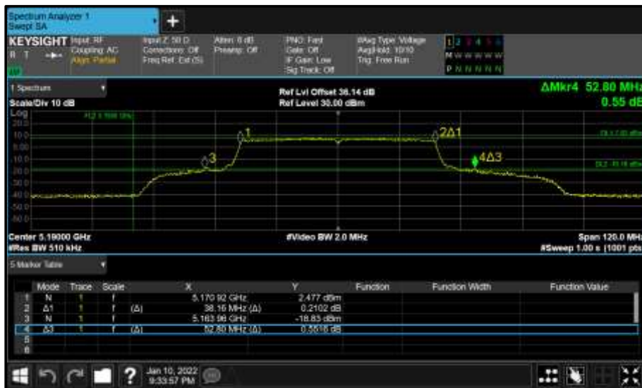
Figure 220 - Core 1 (B) 5190 MHz (CH38) 26 dB and 99% Bandwidth
