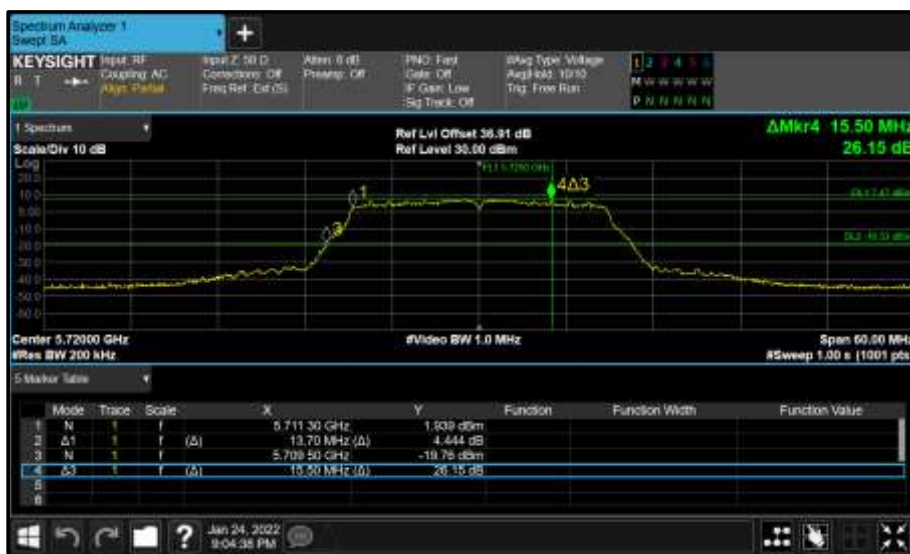
Figure 402 - Core 1 (B) 5720 MHz (CH144) 26 dB and 99% Bandwidth
