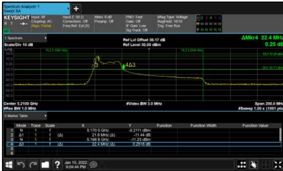
Figure 263 - Core 0 (A) 5210 MHz (CH42) 26 dB and 99% Bandwidth
