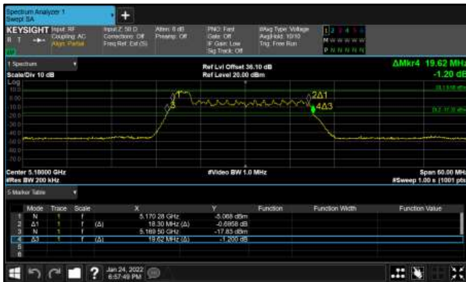
Figure 200 - Core 1 (B) 5180 MHz (CH36) 26 dB and 99% Bandwidth
