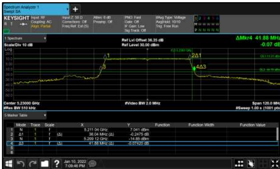
Figure 218 - Core 1 (B) 5230 MHz (CH46) 26 dB and 99% Bandwidth
