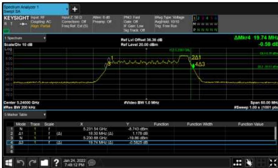
Figure 210 - Core 1 (B) 5240 MHz (CH48) 26 dB and 99% Bandwidth
