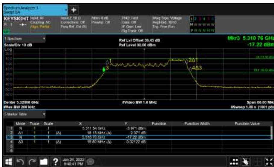
Figure 343 - Core 1 (B) 5320 MHz (CH64) 26 dB and 99% Bandwidth
