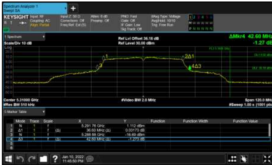
Figure 303 - Core 0 (A) 5310 MHz (CH62) 26 dB and 99% Bandwidth
