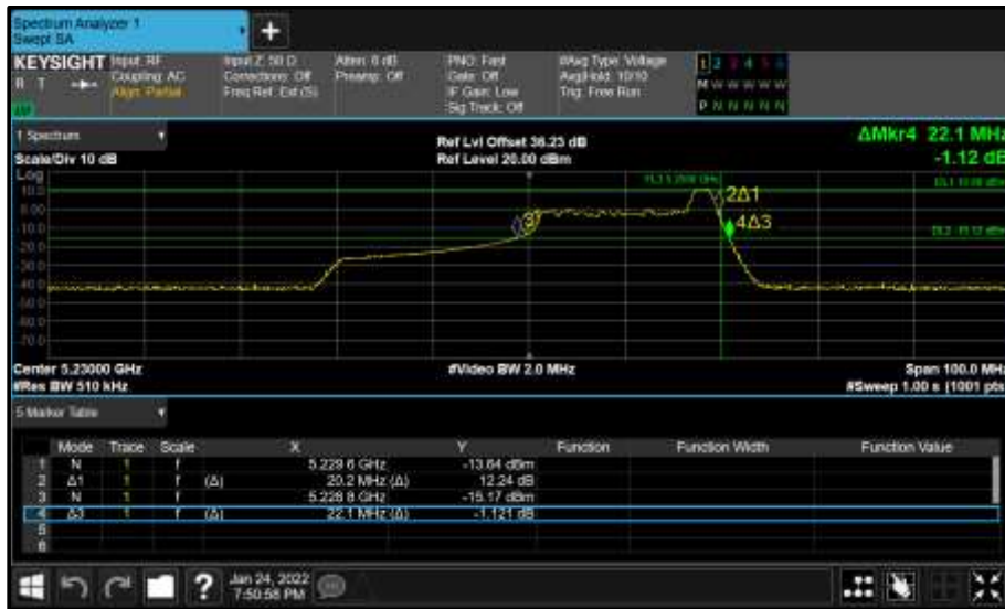
Figure 249 - Core 0 (A) 5230 MHz (CH46) 26 dB and 99% Bandwidth
