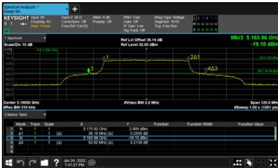
Figure 228 - Core 1 (B) 5190 MHz (CH38) 26 dB and 99% Bandwidth
