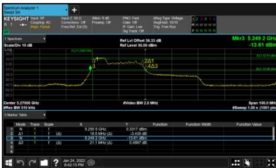
Figure 361 - Core 1 (B) 5270 MHz (CH54) 26 dB and 99% Bandwidth
