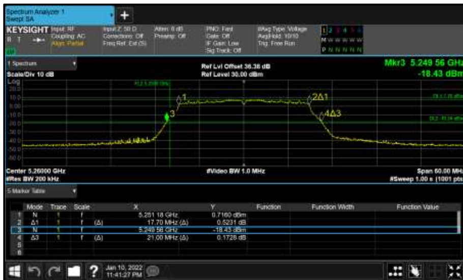
Figure 288 - Core 1 (B) 5260 MHz (CH52) 26 dB and 99% Bandwidth
