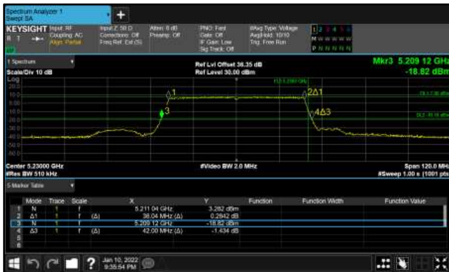
Figure 222 - Core 1 (B) 5230 MHz (CH46) 26 dB and 99% Bandwidth
