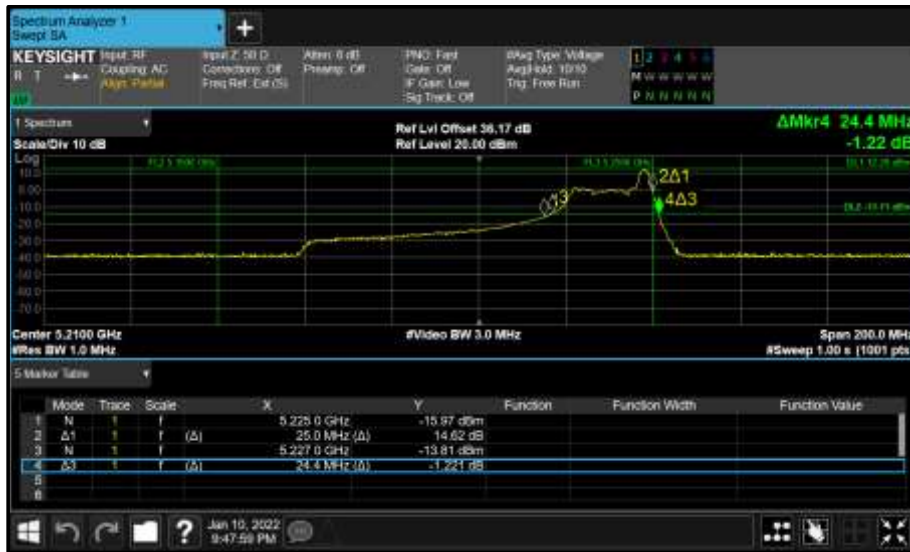
Figure 271 - Core 0 (A) 5210 MHz (CH42) 26 dB and 99% Bandwidth
