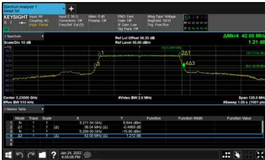
Figure 226 - Core 1 (B) 5230 MHz (CH46) 26 dB and 99% Bandwidth
