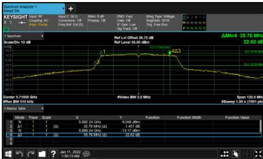
Figure 406 - Core 0 (A) 5710 MHz (CH142) 26 dB and 99% Bandwidth
