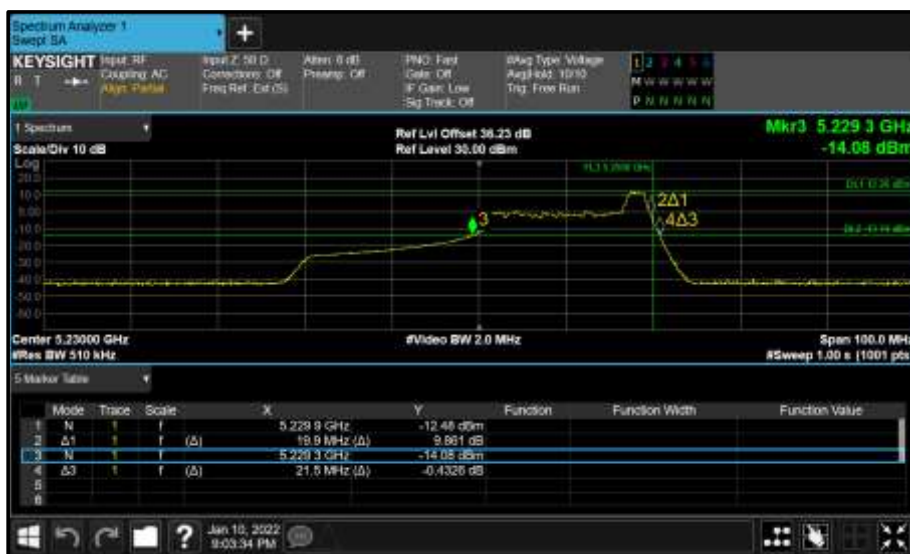
Figure 234 - Core 0 (A) 5230 MHz (CH46) 26 dB and 99% Bandwidth
