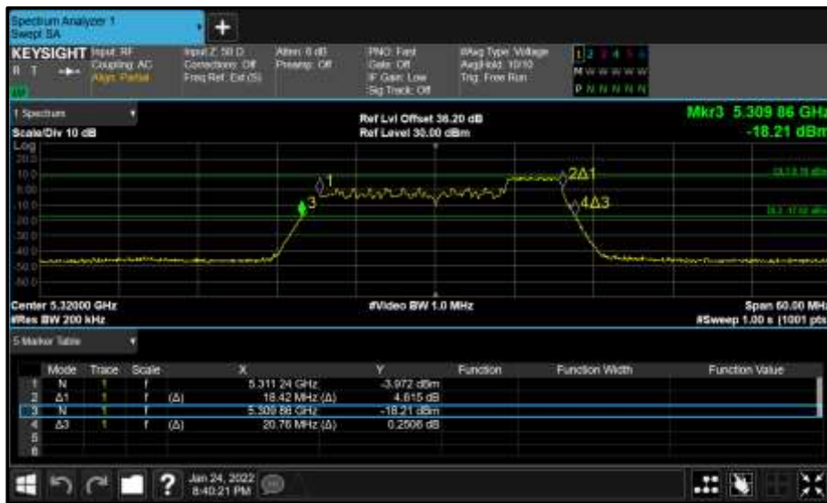
Figure 342 - Core 0 (A) 5320 MHz (CH64) 26 dB and 99% Bandwidth
