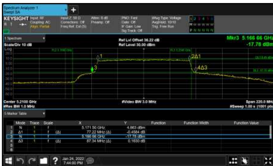
Figure 260 - Core 1 (B) 5210 MHz (CH42) 26 dB and 99% Bandwidth
