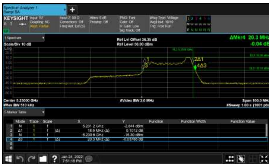
Figure 250 - Core 1 (B) 5230 MHz (CH46) 26 dB and 99% Bandwidth
