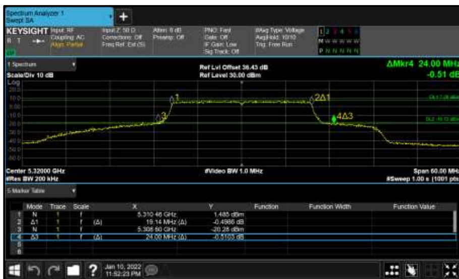
Figure 322 - Core 1 (B) 5320 MHz (CH64) 26 dB and 99% Bandwidth
