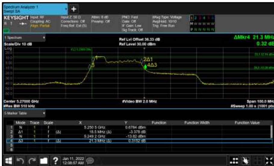
Figure 357 - Core 1 (B) 5270 MHz (CH54) 26 dB and 99% Bandwidth
