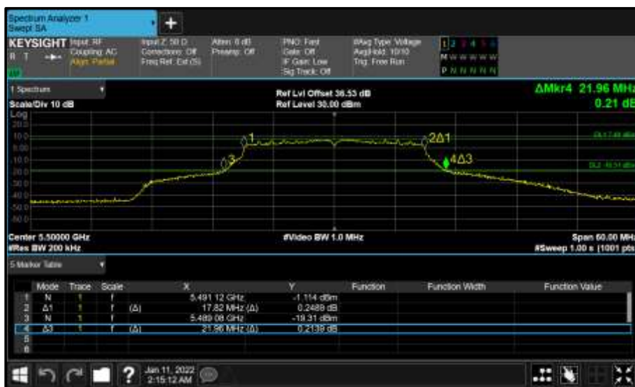
Figure 388 - Core 1 (B) 5500 MHz (CH100) 26 dB and 99% Bandwidth
