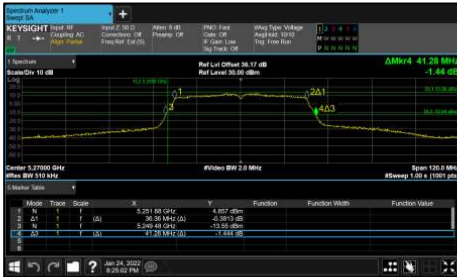
Figure 305 - Core 0 (A) 5270 MHz (CH54) 26 dB and 99% Bandwidth
