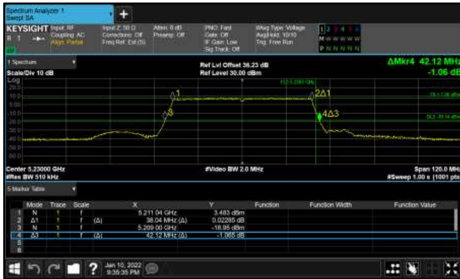
Figure 221 - Core 0 (A) 5230 MHz (CH46) 26 dB and 99% Bandwidth
