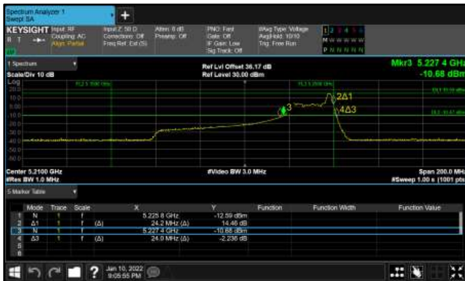
Figure 264 - Core 0 (A) 5210 MHz (CH42) 26 dB and 99% Bandwidth
