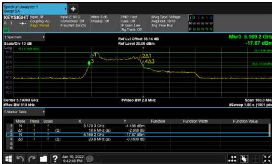
Figure 240 - Core 1 (B) 5190 MHz (CH38) 26 dB and 99% Bandwidth
