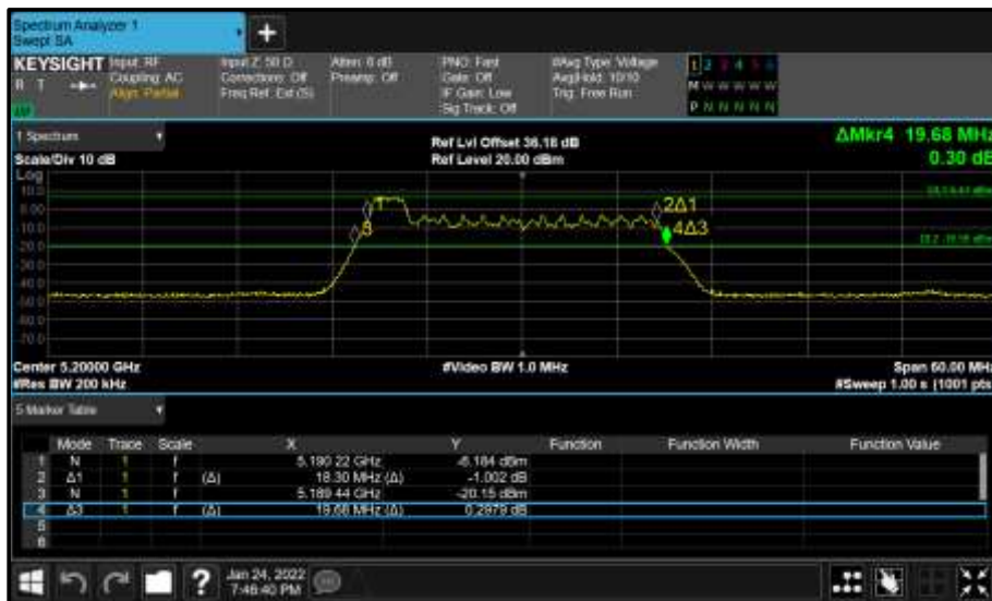
Figure 208 - Core 1 (B) 5200 MHz (CH40) 26 dB and 99% Bandwidth
