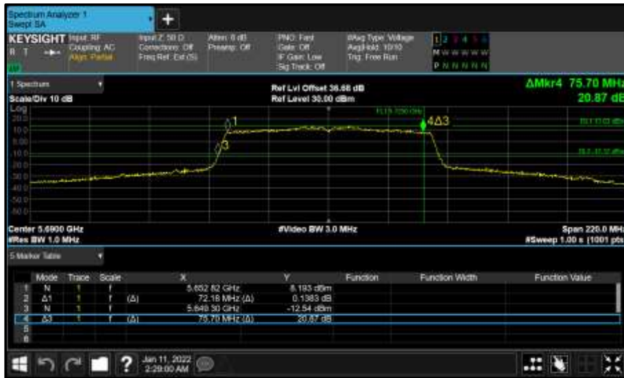
Figure 430 - Core 0 (A) 5690 MHz (CH138) 26 dB and 99% Bandwidth
