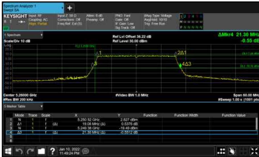
Figure 317 - Core 0 (A) 5260 MHz (CH52) 26 dB and 99% Bandwidth
