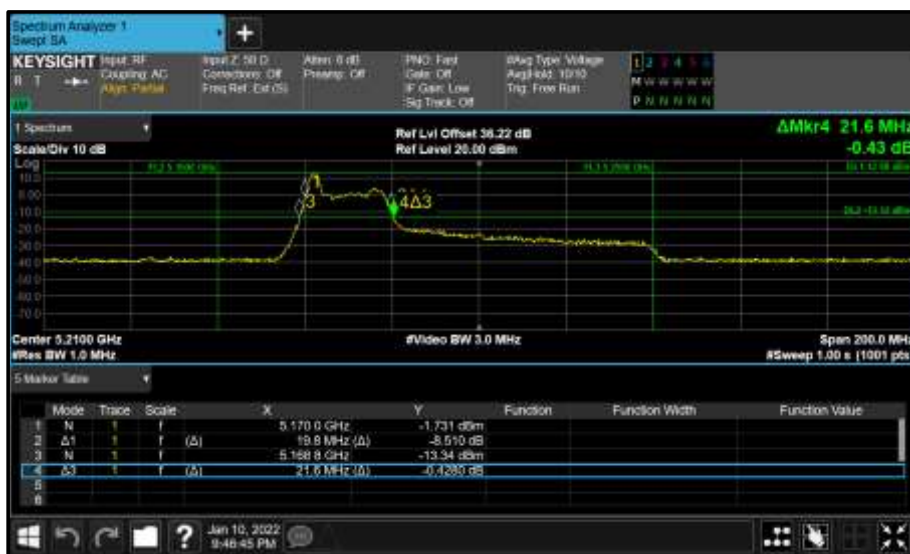
Figure 270 - Core 1 (B) 5210 MHz (CH42) 26 dB and 99% Bandwidth
