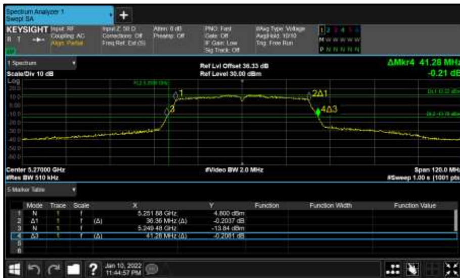
Figure 302 - Core 1 (B) 5270 MHz (CH54) 26 dB and 99% Bandwidth
