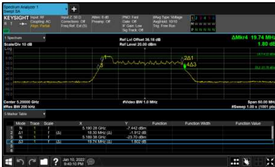
Figure 196 - Core 1 (B) 5200 MHz (CH40) 26 dB and 99% Bandwidth
