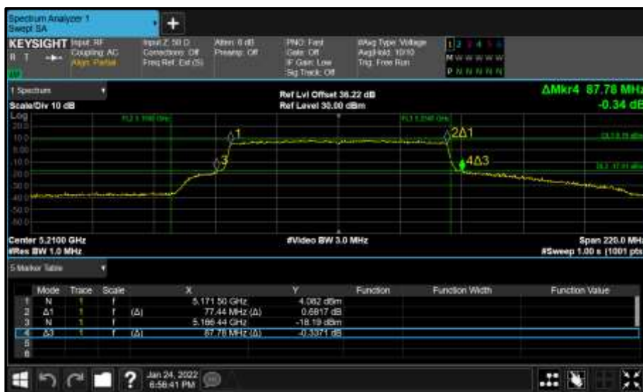
Figure 258 - Core 1 (B) 5210 MHz (CH42) 26 dB and 99% Bandwidth
