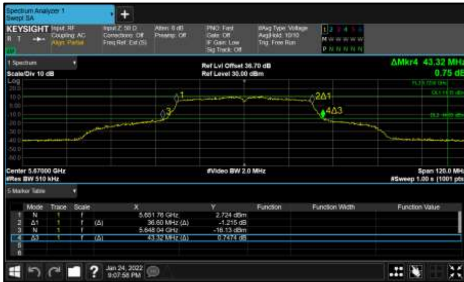
Figure 419 - Core 0 (A) 5670 MHz (CH134) 26 dB and 99% Bandwidth
