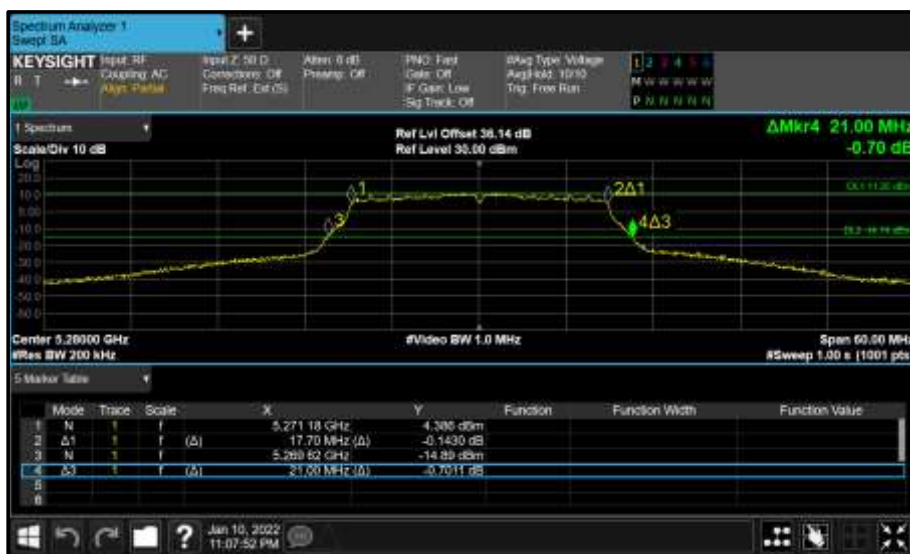
Figure 285 - Core 0 (A) 5280 MHz (CH56) 26 dB and 99% Bandwidth
