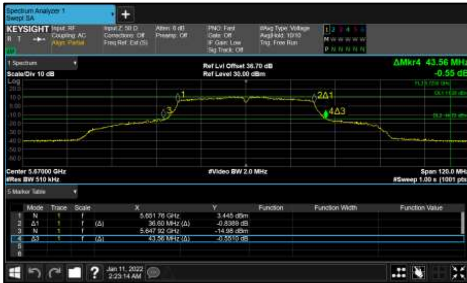
Figure 411 - Core 0 (A) 5670 MHz (CH134) 26 dB and 99% Bandwidth
