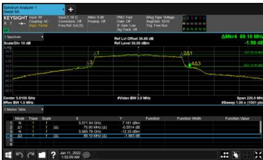
Figure 424 - Core 0 (A) 5610 MHz (CH122) 26 dB and 99% Bandwidth
