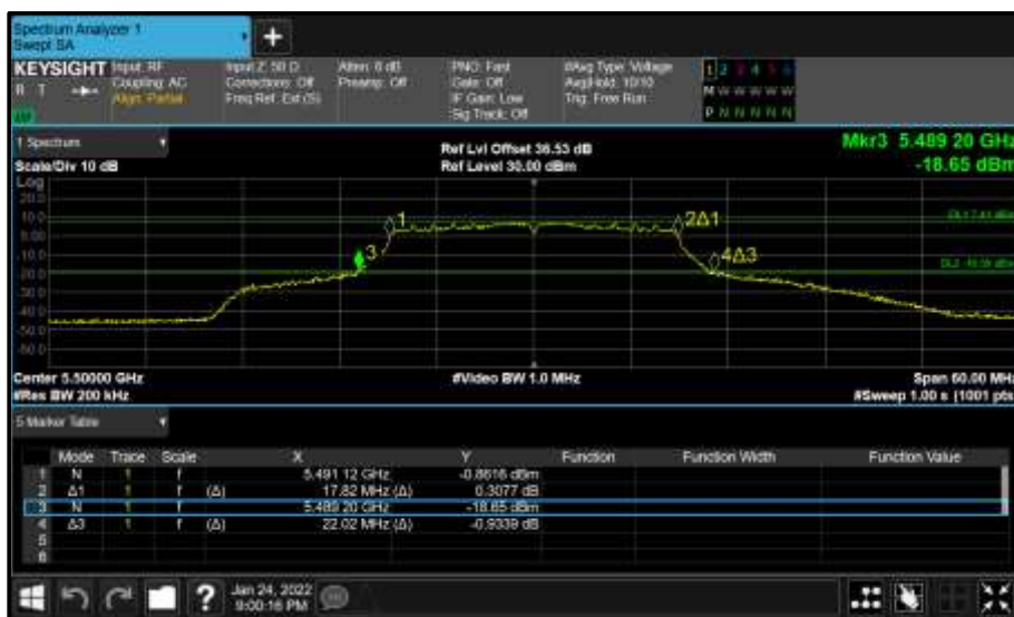
Figure 396 - Core 1 (B) 5500 MHz (CH100) 26 dB and 99% Bandwidth
