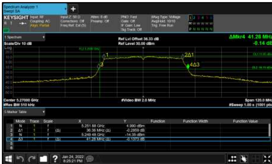
Figure 306 - Core 1 (B) 5270 MHz (CH54) 26 dB and 99% Bandwidth
