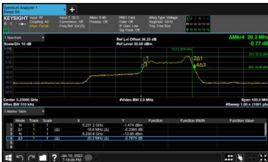
Figure 238 - Core 1 (B) 5230 MHz (CH46) 26 dB and 99% Bandwidth
