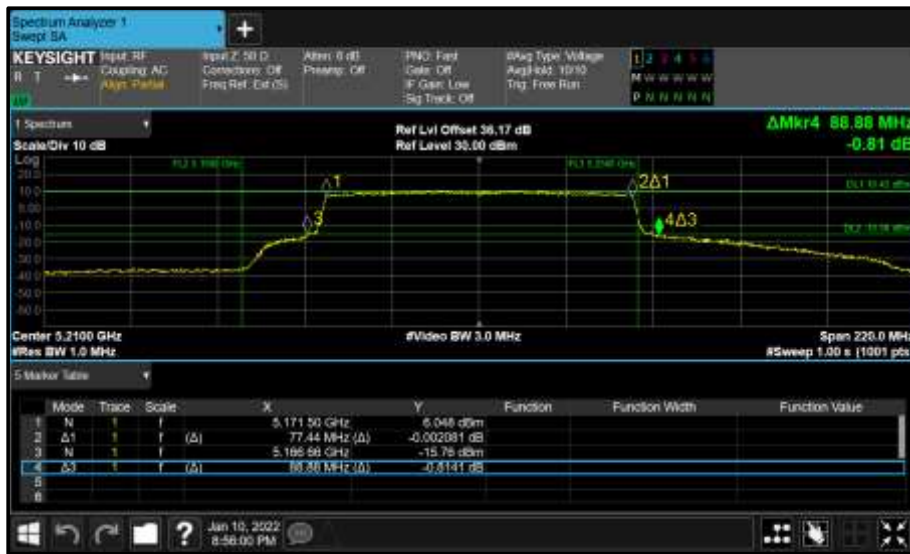
Figure 252 - Core 0 (A) 5210 MHz (CH42) 26 dB and 99% Bandwidth
