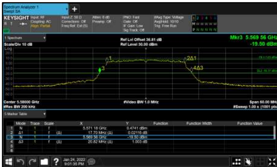
Figure 398 - Core 1 (B) 5580 MHz (CH116) 26 dB and 99% Bandwidth
