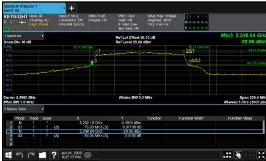
Figure 312 - Core 0 (A) 5290 MHz (CH58) 26 dB and 99% Bandwidth
