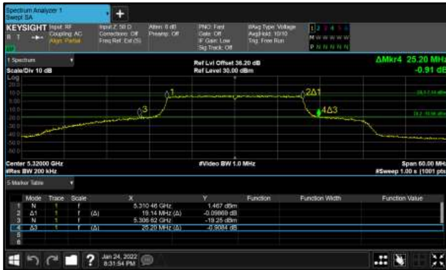
Figure 327 - Core 0 (A) 5320 MHz (CH64) 26 dB and 99% Bandwidth
