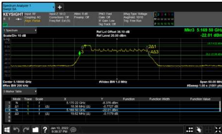
Figure 194 - Core 1 (B) 5180 MHz (CH36) 26 dB and 99% Bandwidth
