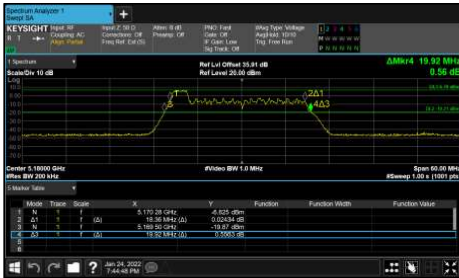
Figure 205 - Core 0 (A) 5180 MHz (CH36) 26 dB and 99% Bandwidth
