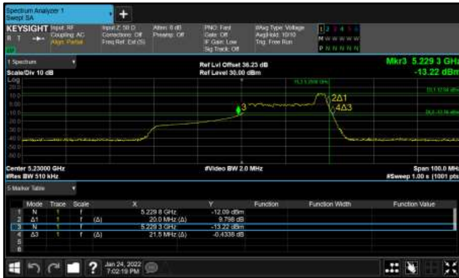
Figure 245 - Core 0 (A) 5230 MHz (CH46) 26 dB and 99% Bandwidth
