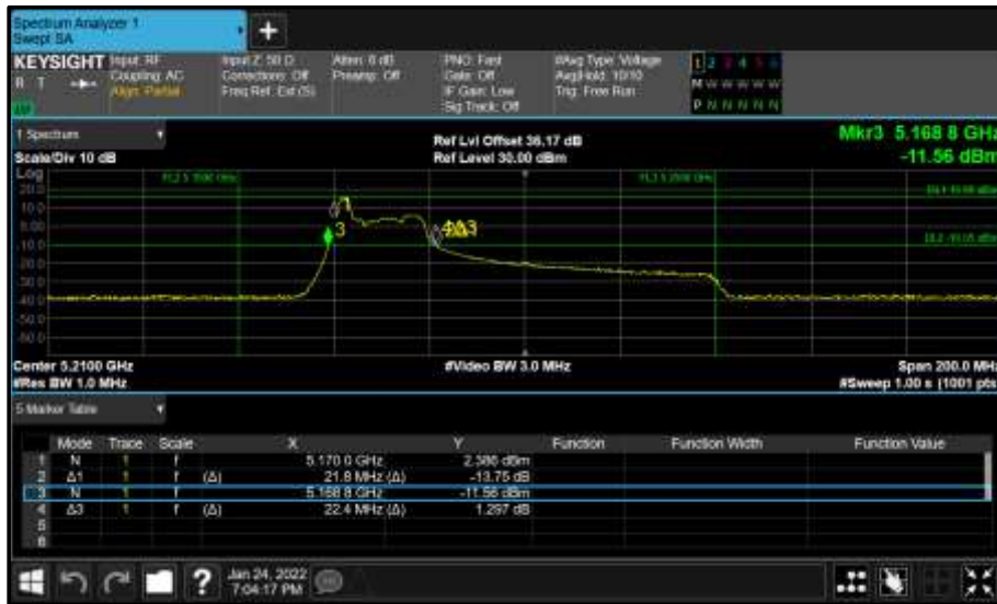
Figure 273 - Core 0 (A) 5210 MHz (CH42) 26 dB and 99% Bandwidth
