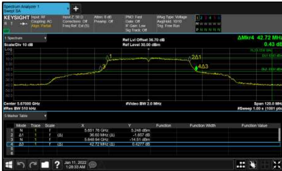
Figure 405 - Core 0 (A) 5670 MHz (CH134) 26 dB and 99% Bandwidth
