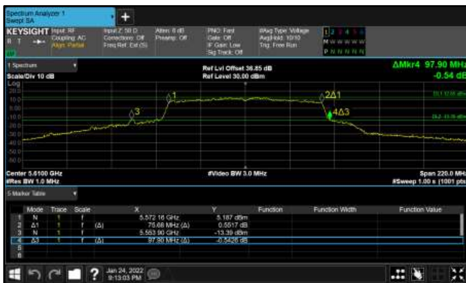
Figure 435 - Core 1 (B) 5610 MHz (CH122) 26 dB and 99% Bandwidth
