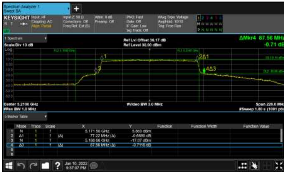
Figure 255 - Core 0 (A) 5210 MHz (CH42) 26 dB and 99% Bandwidth
