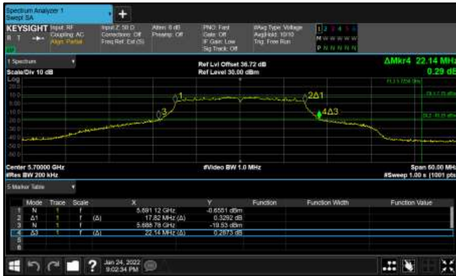
Figure 399 - Core 0 (A) 5700 MHz (CH140) 26 dB and 99% Bandwidth
