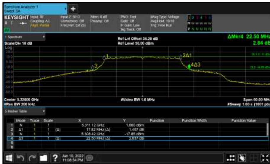
Figure 286 - Core 0 (A) 5320 MHz (CH64) 26 dB and 99% Bandwidth
