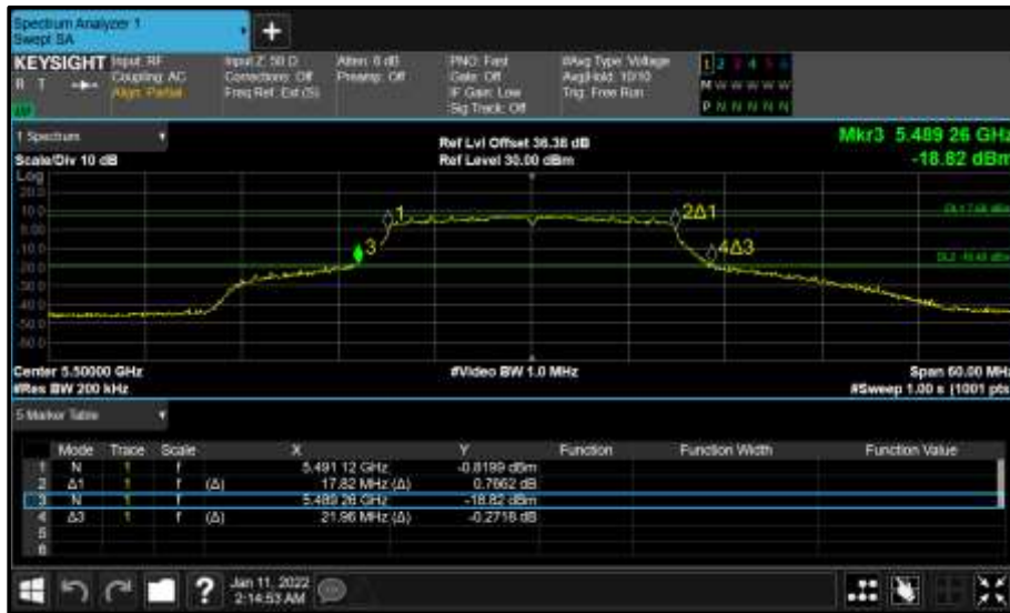
Figure 387 - Core 0 (A) 5500 MHz (CH100) 26 dB and 99% Bandwidth
