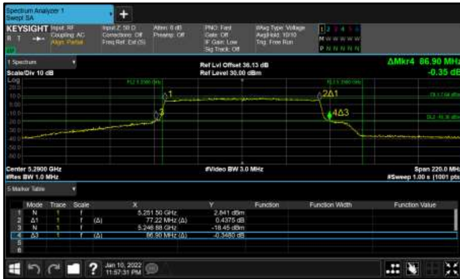
Figure 365 - Core 0 (A) 5290 MHz (CH58) 26 dB and 99% Bandwidth
