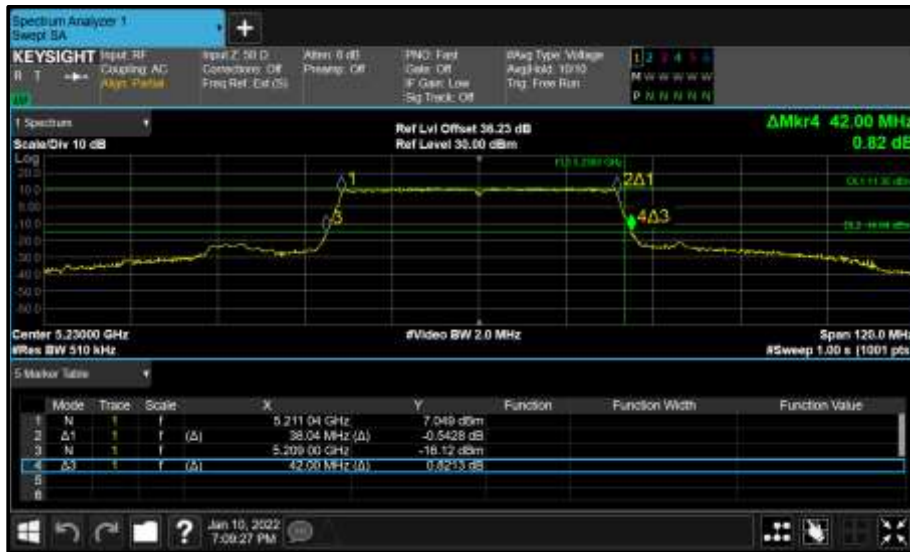
Figure 217 - Core 0 (A) 5230 MHz (CH46) 26 dB and 99% Bandwidth
