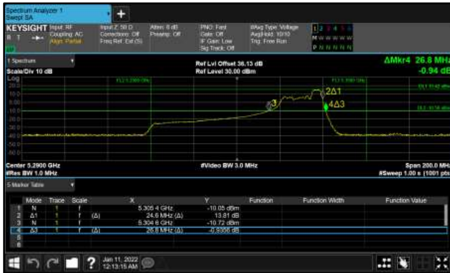
Figure 373 - Core 0 (A) 5290 MHz (CH58) 26 dB and 99% Bandwidth
