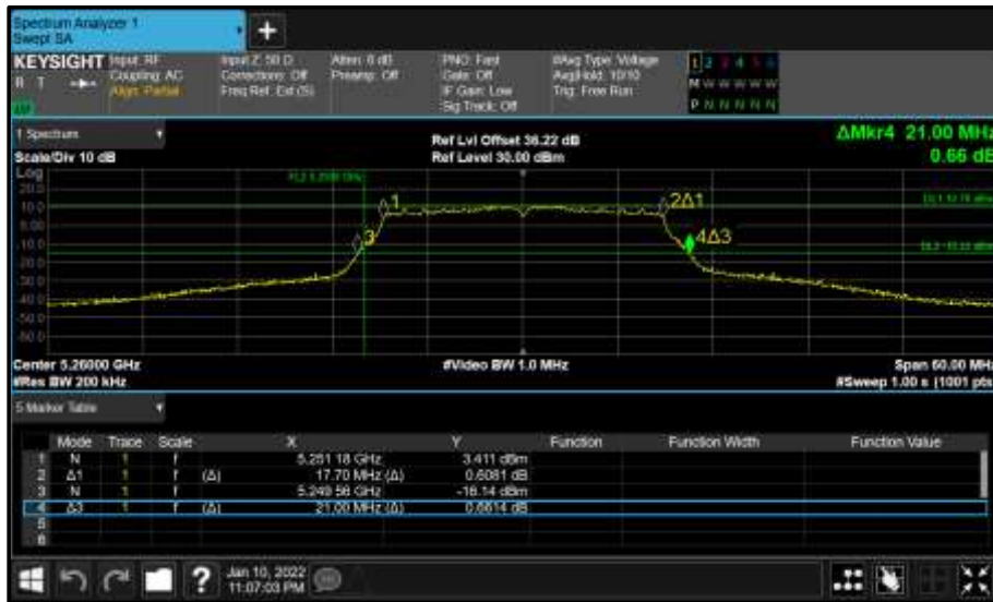
Figure 284 - Core 0 (A) 5260 MHz (CH52) 26 dB and 99% Bandwidth
