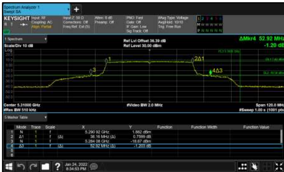
Figure 353 - Core 1 (B) 5310 MHz (CH62) 26 dB and 99% Bandwidth
