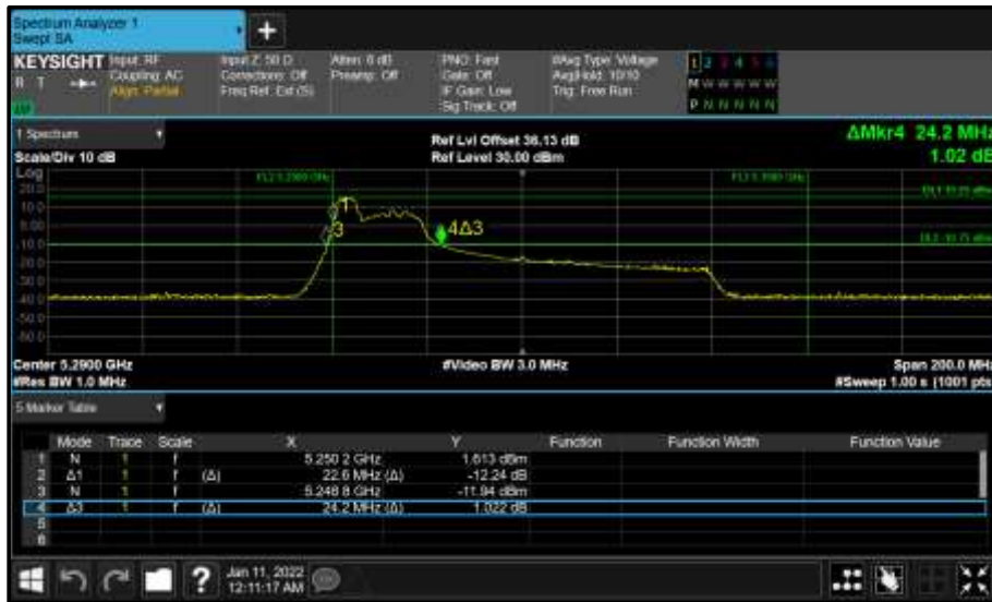
Figure 371 - Core 0 (A) 5290 MHz (CH58) 26 dB and 99% Bandwidth
