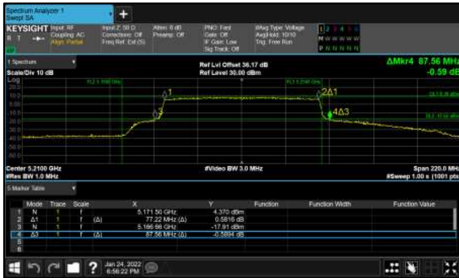
Figure 257 - Core 0 (A) 5210 MHz (CH42) 26 dB and 99% Bandwidth
