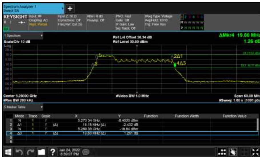
Figure 341 - Core 1 (B) 5280 MHz (CH56) 26 dB and 99% Bandwidth
