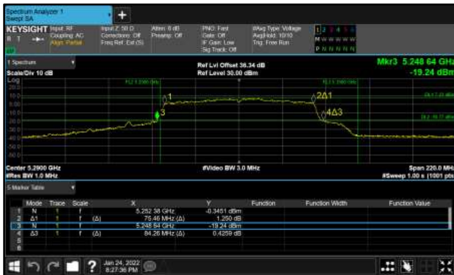
Figure 313 - Core 1 (B) 5290 MHz (CH58) 26 dB and 99% Bandwidth
