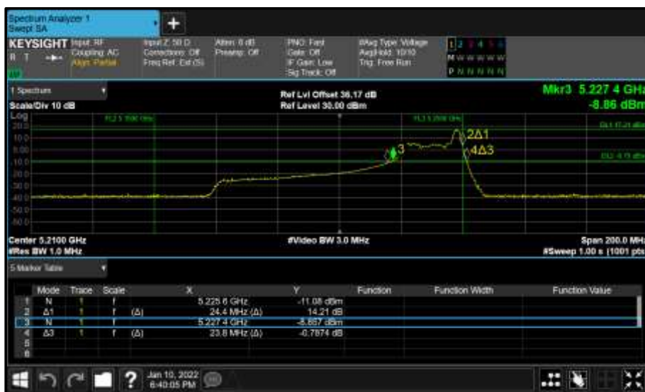
Figure 262 - Core 0 (A) 5210 MHz (CH42) 26 dB and 99% Bandwidth
