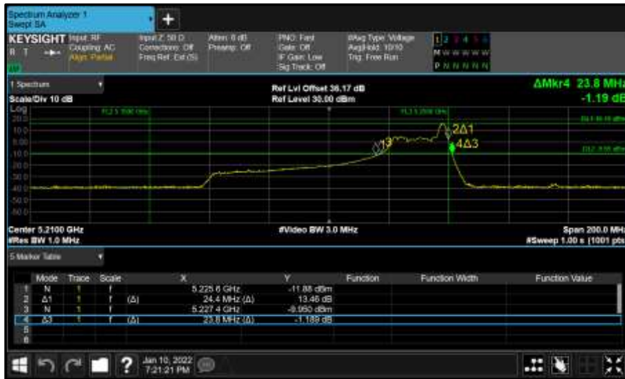
Figure 267 - Core 0 (A) 5210 MHz (CH42) 26 dB and 99% Bandwidth
