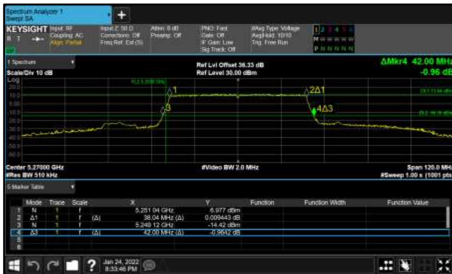
Figure 351 - Core 1 (B) 5270 MHz (CH54) 26 dB and 99% Bandwidth
