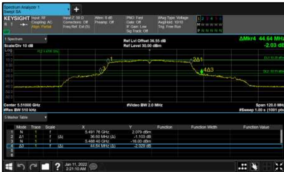
Figure 408 - Core 1 (B) 5510 MHz (CH102) 26 dB and 99% Bandwidth
