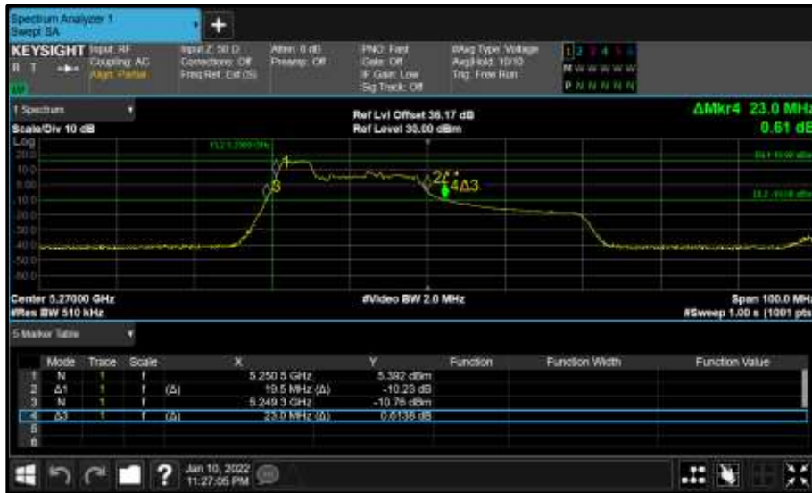
Figure 354 - Core 0 (A) 5270 MHz (CH54) 26 dB and 99% Bandwidth
