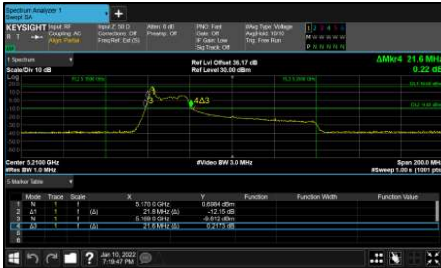
Figure 265 - Core 0 (A) 5210 MHz (CH42) 26 dB and 99% Bandwidth
