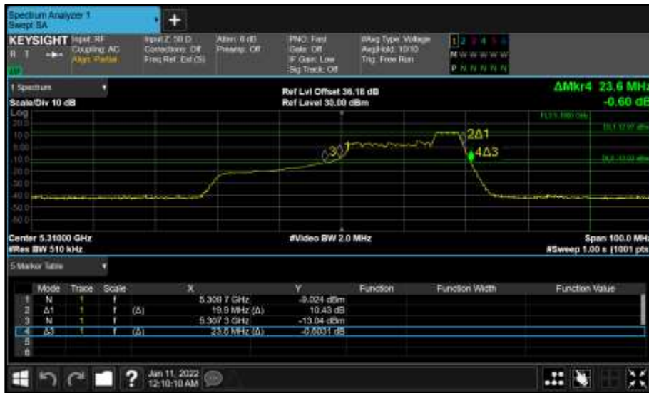
Figure 358 - Core 0 (A) 5310 MHz (CH62) 26 dB and 99% Bandwidth
