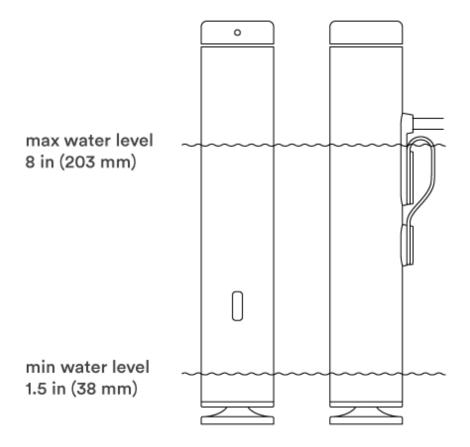
However, you can always use the clip to attach Joule to the rim of your container and increase the maximum water level, as demonstrated in the photo below.
