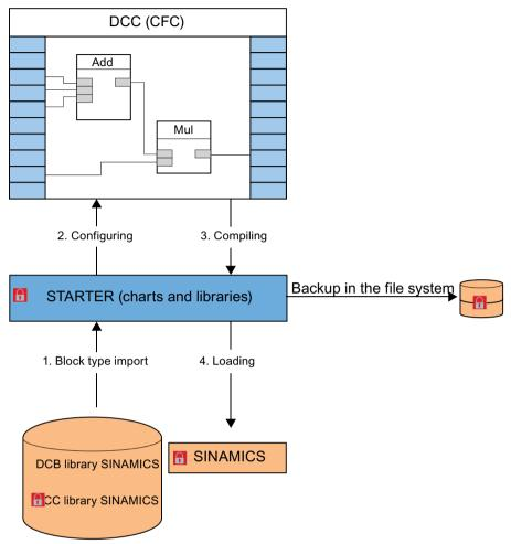
Figure 7-11 Flow of configuration data: Example for DCC Classic V2.1 ... V3.4 (STARTER)
