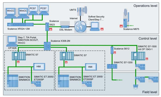
Figure 7-4 Display of a typical production plant with protected areas
