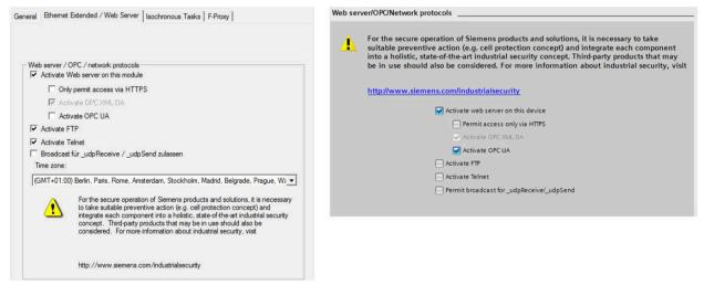
Figure 7-8 Activating the SIMOTION IT Web server functions in SIMOTION SCOUT or SIMOTION SCOUT TIA
