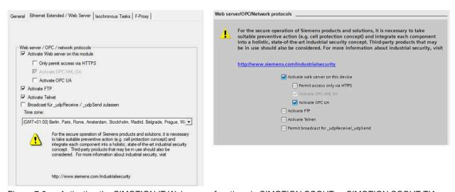
Figure 7-9 Activating the SIMOTION IT Web server functions in SIMOTION SCOUT or SIMOTION SCOUT TIA
