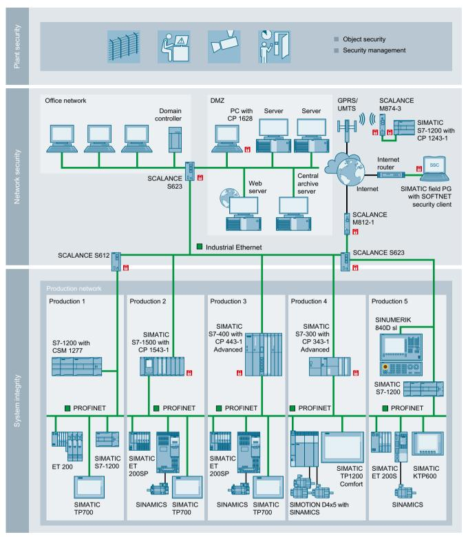
Figure 6-2 SCALANCE S application example
