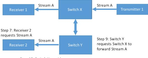
Step 10: Switch Y provides Receiver 2 Stream A
