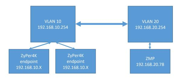
The ZyPer4K Endpoints are located on VLAN 10 and the 192.168.10.X subnet. The ZyPer Management Platform is on VLAN 20 and the 192.168.20.X subnet.
