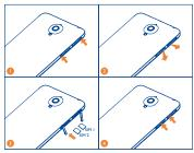
Hold the phone securely with the front facing down. Then press the spot on the cover of slot I for it to open. Gently move the cover to fully expose the slot. Insert SIM I with its chip facing up and close the cover with your thumb.
