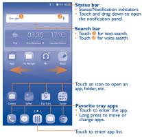
The Home screen is provided in an extended format to allow more space for adding apps, shortcuts etc. Slide the Home screen left and right to get a complete view.
