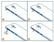
Hold the phone securely with the front facing down. Then press the spot on the microSD slot for it to open. Gently move the cover to fully expose the slot. Insert the microSD with its chip facing up and close the cover with your thumb.
