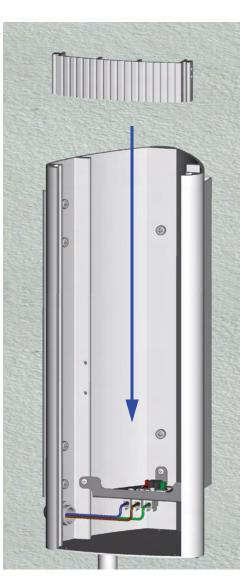
Re-attach bonding wire and tighten screw.
