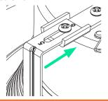
Press both pairs of torsion spring legs together and insert them into the receivers inside the housing.
