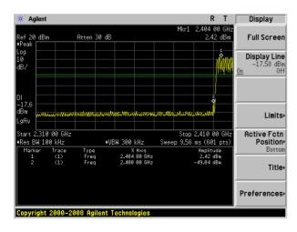
GFSK: Band Edge-High Channel (Hopping Mode)
