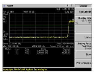
8-DPSK: Band Edge-High Channel (Hopping Mode)
