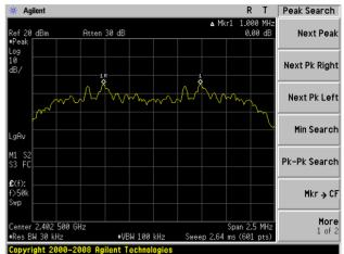
(1Mbps) Channel Separation plot on channel 39-40
