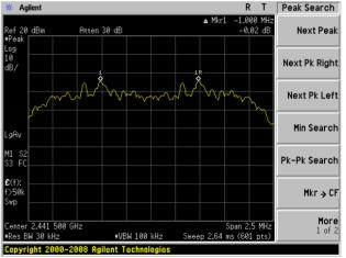
(1Mbps) Channel Separation plot on channel 77-78
