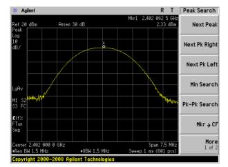
Peak output Power plot on channel 00 (2Mbps)
