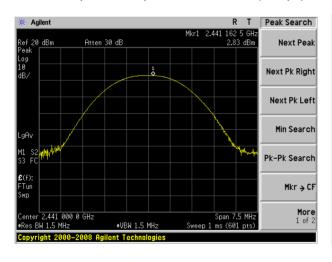
Peak output Power plot on channel 39 (2Mbps)
