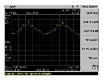
(2Mbps) Channel Separation plot on channel 39-40
