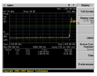
$\pi$  /4-DQPSK: Band Edge-High Channel (Hopping Mode)
