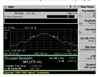
20dB Bandwidth plot on channel 78 (2Mbps)
