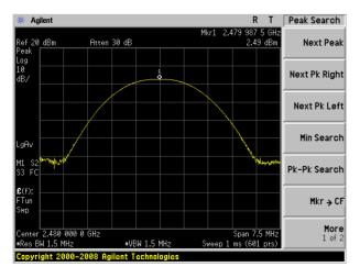
Peak output Power plot on channel 78 (2Mbps)
