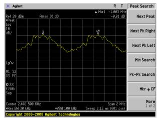
(2Mbps) Channel Separation plot on channel 00-01
