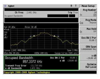
20dB Bandwidth plot on channel 39 (2Mbps)
