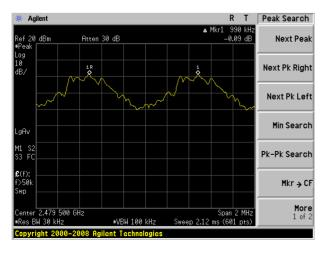
(2Mbps) Channel Separation plot on channel 77-78
