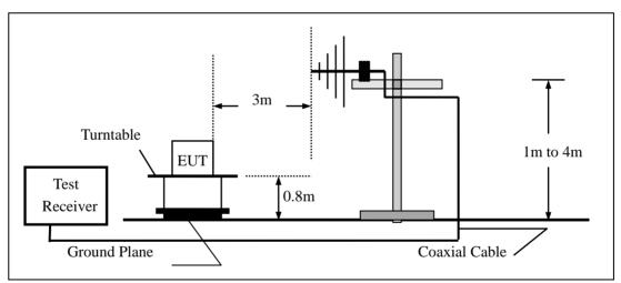
(c) For radiated emissions above 1000MHz
