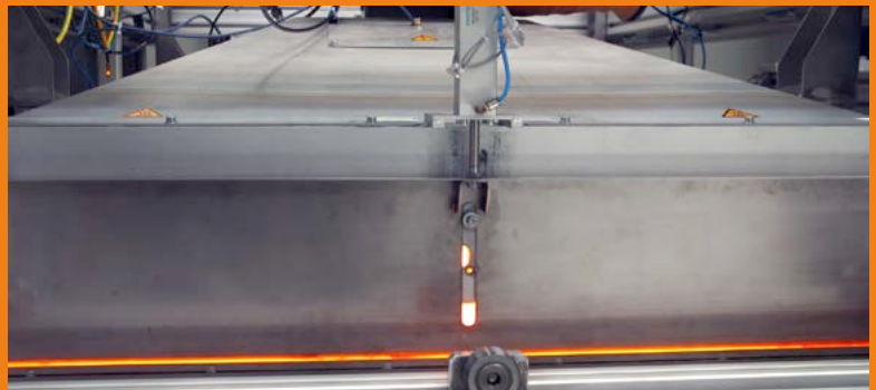
Dieffenbacher GmbH - fastest tape laying system in the world achieves high product quality through consolidation
