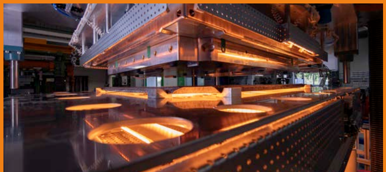
Vesper GmbH & Co. KG - hot solution for cool automotive interiors: laminating-edge-folding system without sliders
