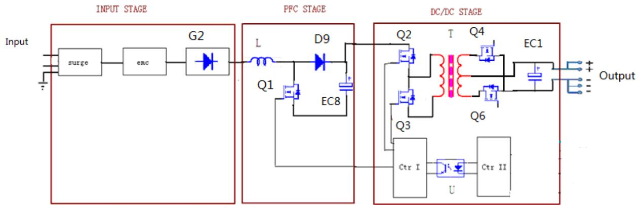
The power supply unit consists of input stage, PFC stage, DC/DC stage, and control circuit. Input stage includes surge protect circuit, EMC circuit, soft-start-up circuit, etc. This circuits help to meet EMC regular of EN55022 etc. DC/DC stage delivers a desired output voltage. Control circuit carries out many functions as OVP, OLP, OTP, loop control.
