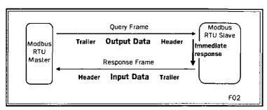
Fig. 2 Shows the MODBUS RTU data exchange.
