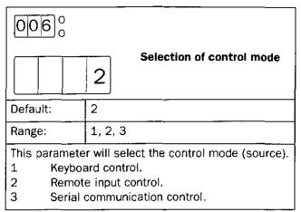
In all control modes it is possible to read out all the information in the soft starter via serial communication, both parameters and view information.
