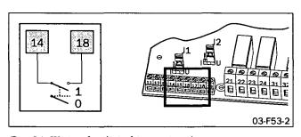
Fig. 54 Wiring for digital input signal.
