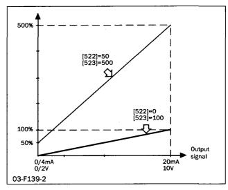
Fig. 60 Scaling of analogue output
