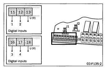
Fig. 57 Wiring for digital inputs 1-4.
