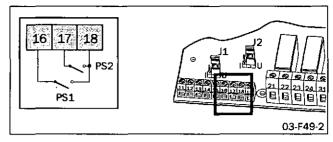
Fig. 67 Connection of external control inputs.
