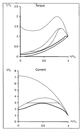
Fig. 10 Soft starting - torque control
