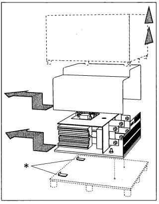
Fig. 2 Unpacking MSF-310 and larger models.
