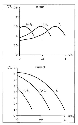
Fig. 12 Voltage/frequency regulation
