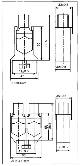
Fig. 72 The terminal clamp.
