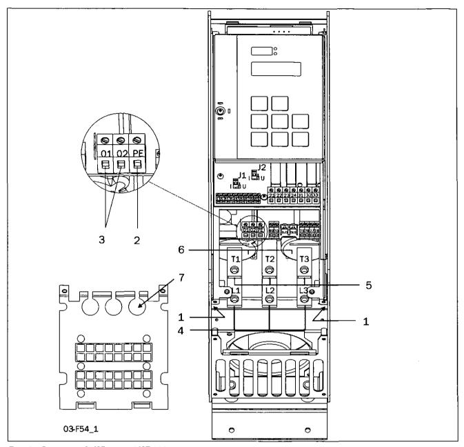
Fig. 19 Connection of MSF-017 to MSF-085.
