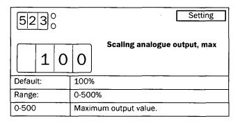
NOTE: The maximum value for scaling the analogue output is reset to the default value 100% if a new output value is chosen in menu [521].
