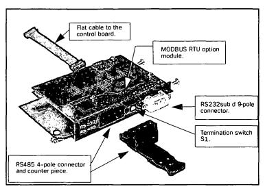
Fig. 13 MODBUS RTU option card.
