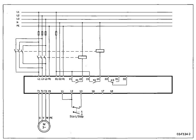
Fig. 45 Reverse current brake wiring example.
