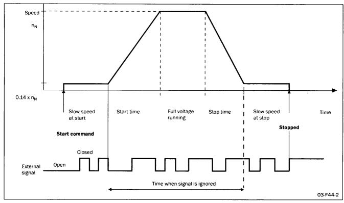
Fig. 46 Slow speed controlled by an external signal.
