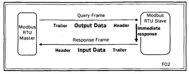
Fig. 2 Shows the MODBUS RTU data exchange.
