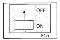
Fig. 13 Termination is ON.
