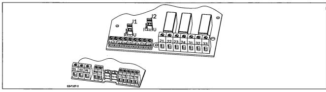
Fig. 23 PCB (control board) connections.
