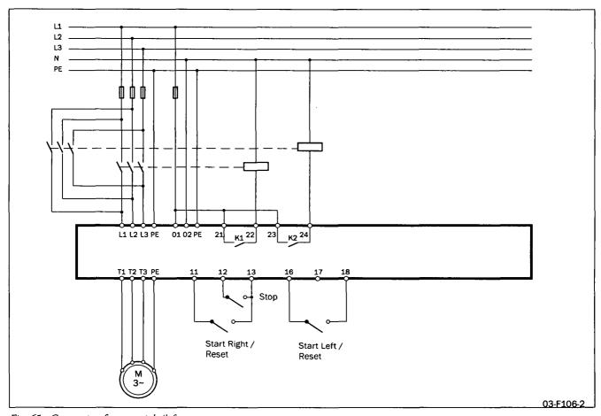
Fig. 65 Connection for start right/left
