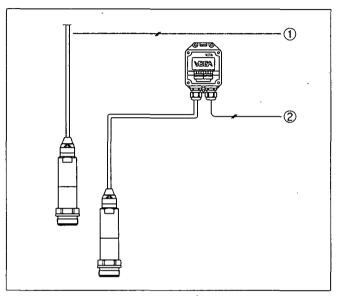
Fig. 3: Connection of VEGABAR 74
