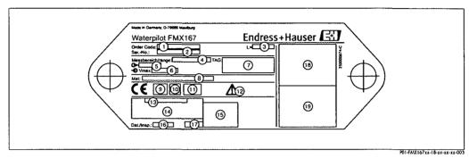
Fig. 1: Nameplate for Waterpilot FMX167
