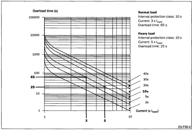
Fig. 34 The thermal curve
