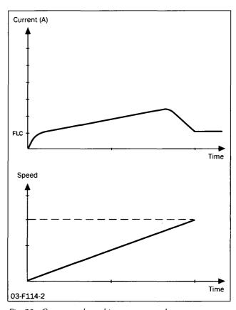
Fig. 38 Current and speed in torque control
