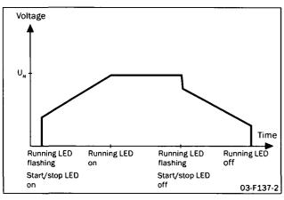
Fig. 33 LED indication at different operation situations.
