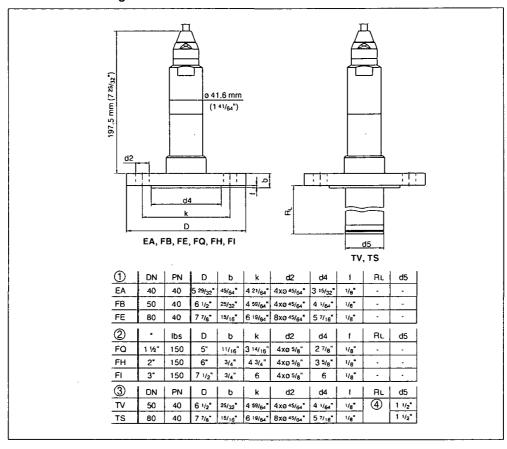
Fig. 15: VEGABAR 74 - flange connection
