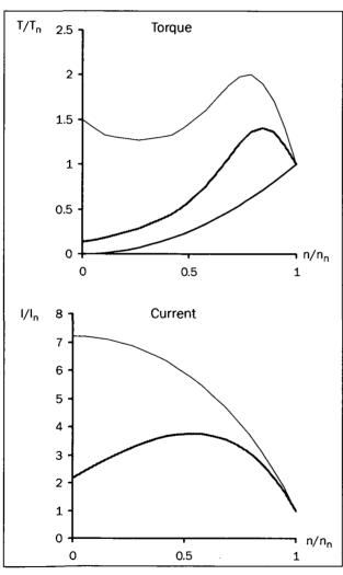
Fig. 8 Soft starting - voltage ramp
