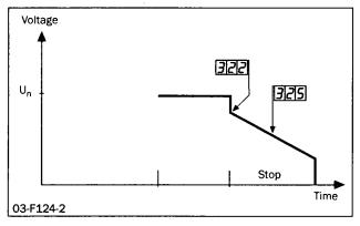
Fig. 44 Menu numbers for step down voltage at stop and stop
