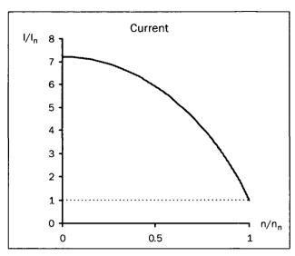
Fig. 4 Typical current characteristics for the DOL start
