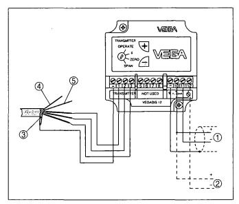
Fig. 6: Terminal assignment, VEGADIS 12
