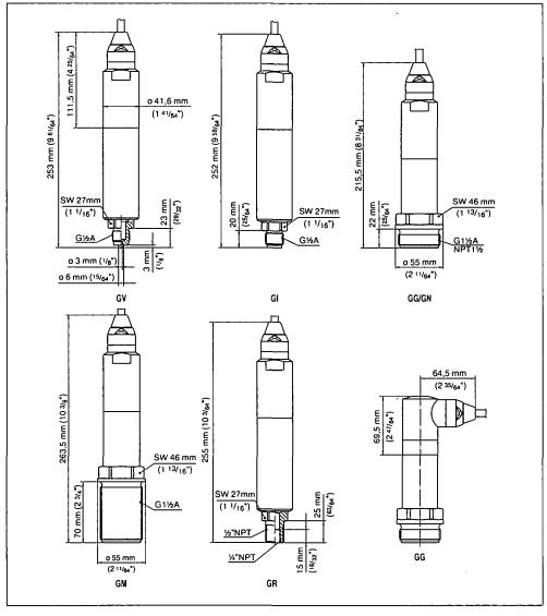
Fig. 12: VEGABAR 74 threaded fitting: GV = G1/2 A manometer connection EN 837, GI = G1/2 A inner G1/2 A, GG = G1/2 A, GN = 11/2 NPT, GM = G1/2 A 70 mm, GR = 1/2 NPT inner 1/2 NPT
