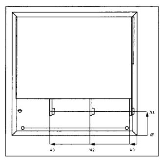
Fig. 16 Busbar distances MSF-310 to MSF-835.
