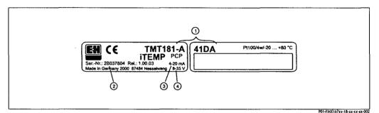
Fig. 3: Nameplate of temperature transmitter TMT181
