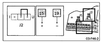
Wiring for analogue output and setting of J2 for analogue current or voltage signal.
