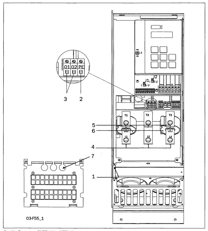
Fig. 20 Connection of MSF-110 to MSF-145.
