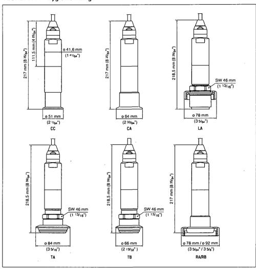
Fig. 13: VEGABAR 74 hygienic litting: CC = Tri-Clamp 1½\*, CA = Tri-Clamp 2\*, LA = hygienic litting with compression nut F40, TA = Tuchenhagen Varivent DN 32, TB = Tuchenhagen Varivent DN 25, RA/RB = bolting DN 40/DN 50 according to DIN 11851
