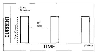
Fig. 30 Duty cycle, bypassed
