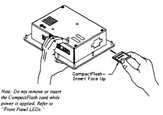
Information stored on a CompactFlash card by a G306A can be read by a card reader attached to a PC. This information is stored in IBM (Windows<sup>©</sup>) PC compatible FAT16 file format.
