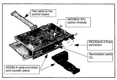
Fig. 4 MODBUS RTU option card.
