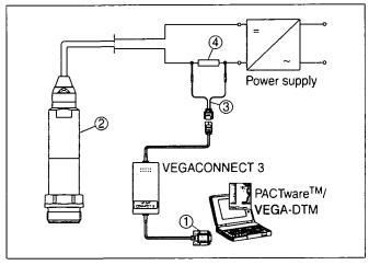
Fig. 8: Connecting the PC to the signal cable
