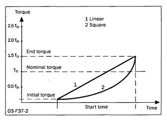
Fig. 37 Torque control at start
