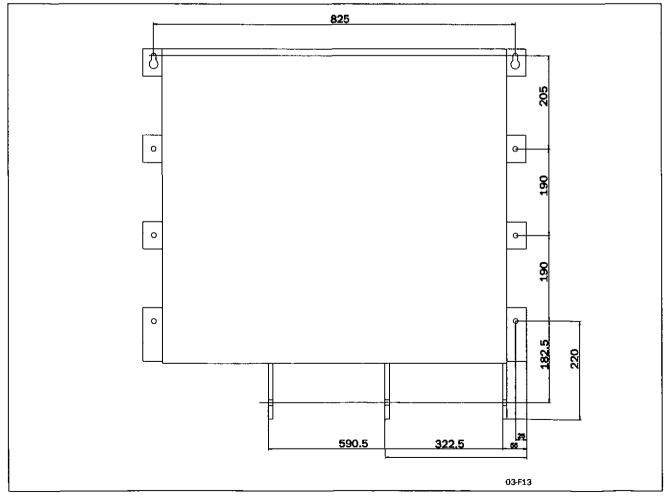
Fig. 18 Hole pattern busbar MSF-1000 to MSF-1400.
