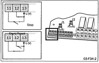
Fig. 64 Connection of terminals for start/stop/reset
