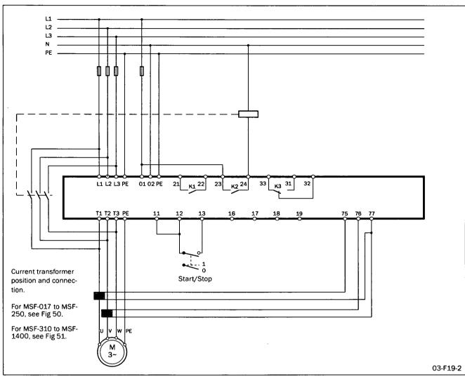
Fig. 49 Bypass wiring example MSF 310-1400.
