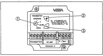
Fig. 7: Adjustment elements of VEGADIS 12
