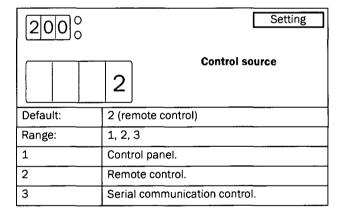
Independent of the chosen control source it is always possible to read out all the information in the softstarter via serial communication, both parameters and view information.
