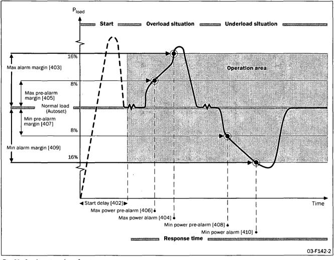
Fig. 52 Load monitor alarm functions
