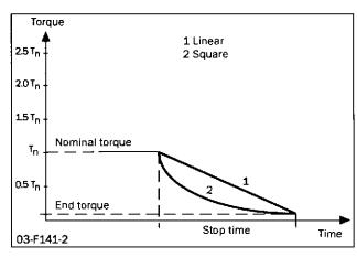
Fig. 43 Torque control at stop
