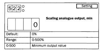
NOTE: The minimum value for scaling the analogue output is reset to the default value 0% if a new output value is chosen in menu [521].
