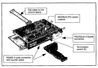
Fig. 4 MODBUS RTU option card.
