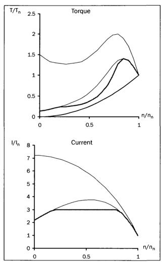
Fig. 9 Soft starting - voltage ramp with current limit
