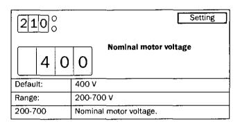
NOTE: Make sure the softstarter's maximum voltage rating is suitable for selected motor voltage.
