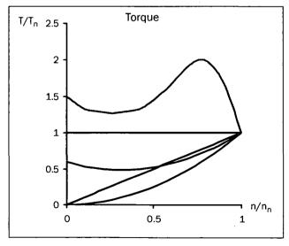
Fig. 5 Typical load torque characteristics
