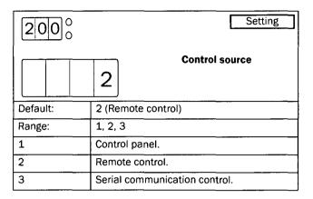
Menu [200] must be set to 1 to be able to operate from control panel.
