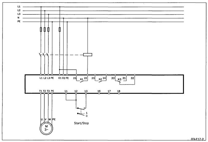
Fig. 25 Standard wiring.
