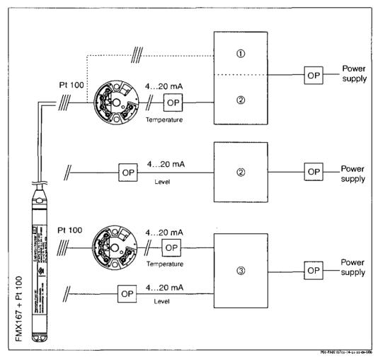
Fig. 13: Wiring up the measuring unit
