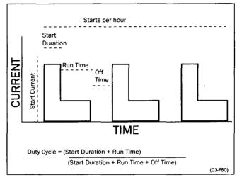
Fig. 28 Duty cycle, non-bypass.
