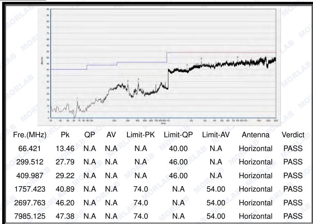
(30MHz to 25GHz, Antenna Horizontal @ GFSK, channel 0)
