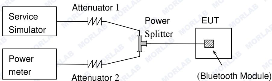
The Bluetooth Module of the EUT is coupled to the Power meter and the Bluetooth Service Simulator (SS) with Attenuators through the Power Splitter; the RF load attached to the EUT antenna terminal is 50Ohm; the path loss as the factor is calibrated to correct the reading. During the measurement, the Bluetooth Module of the EUT is activated and controlled by the SS, and is set to operate under test mode transmitting 339 bytes DH5 packages at maximum power.
