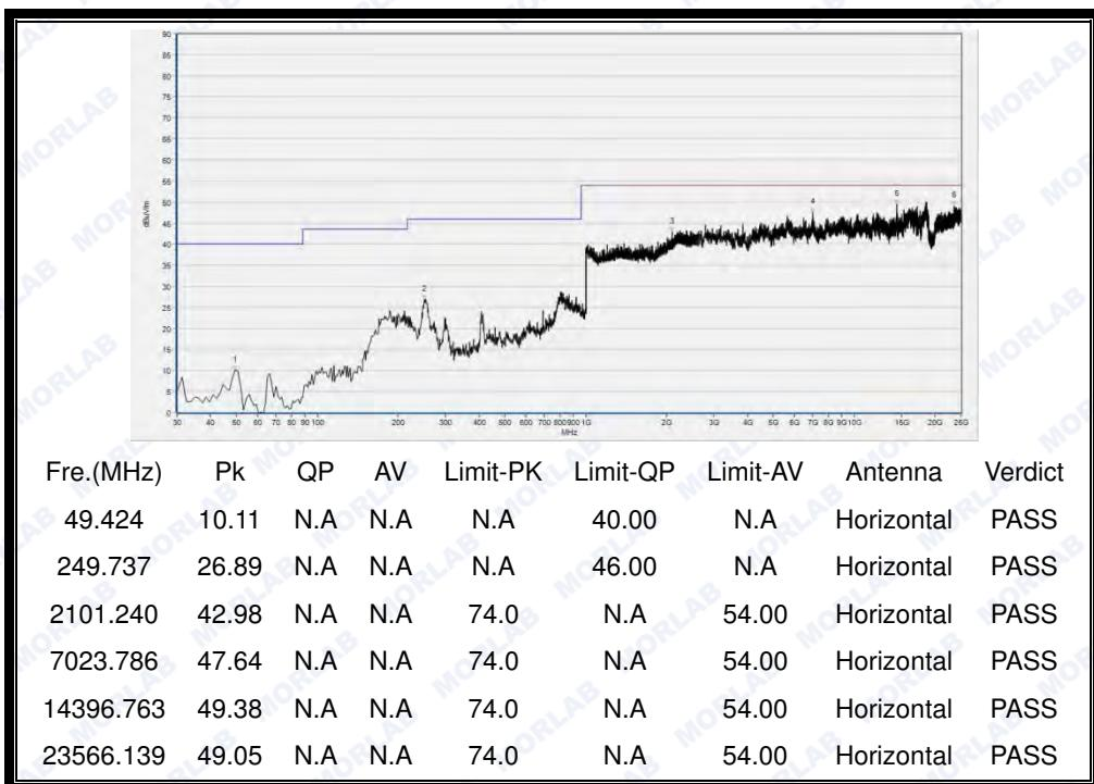
(30MHz to 25GHz, Antenna Horizontal @  $\pi/4$ -DQPSK, channel 78)
