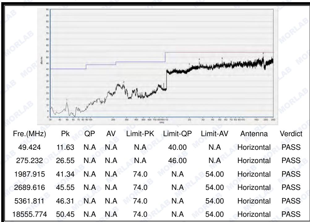
(30MHz to 25GHz, Antenna Horizontal @8-DPSK, channel 78)
