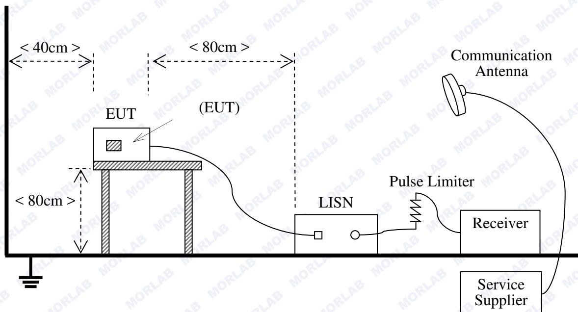
The Table-top EUT was placed upon a non-metallic table 0.8m above the horizontal metal reference ground plane. EUT was connected to LISN and LISN was connected to reference Ground Plane. EUT was 80cm from LISN. The set-up and test methods were according to ANSI C63.4:2014
