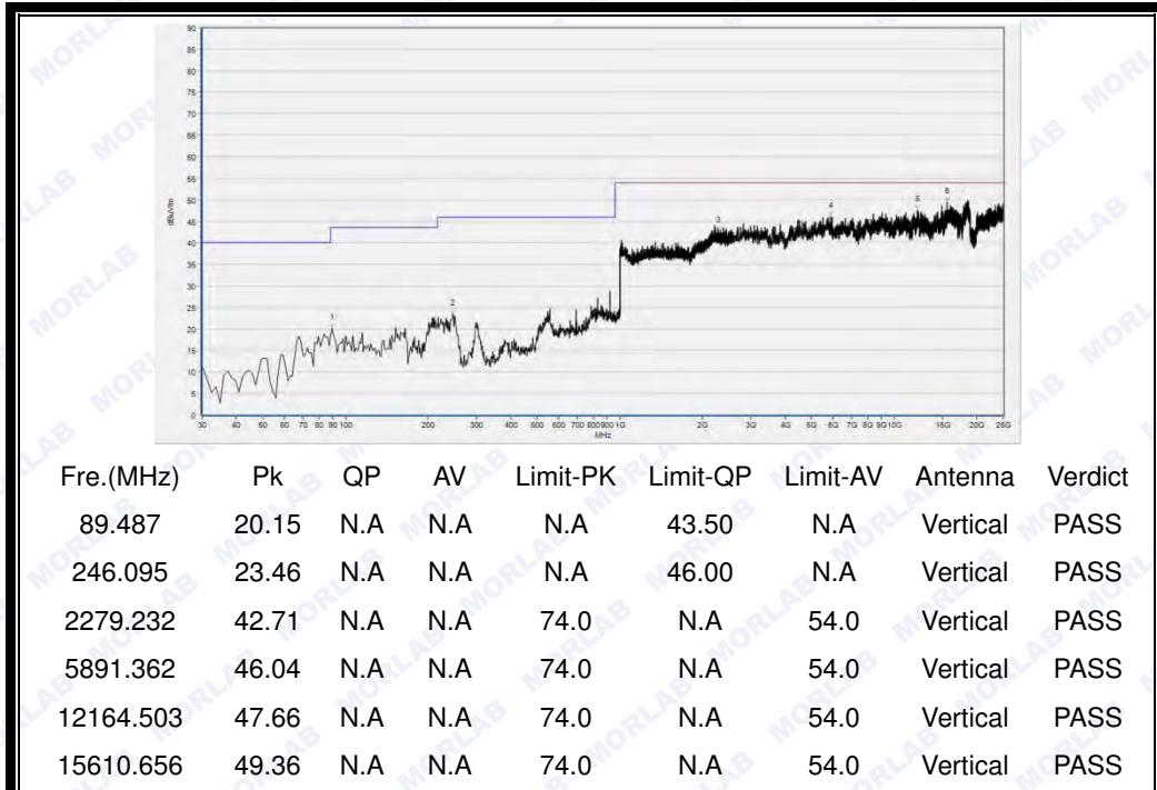
(30MHz to 25GHz, Antenna Vertical @8-DPSK, channel 39)
