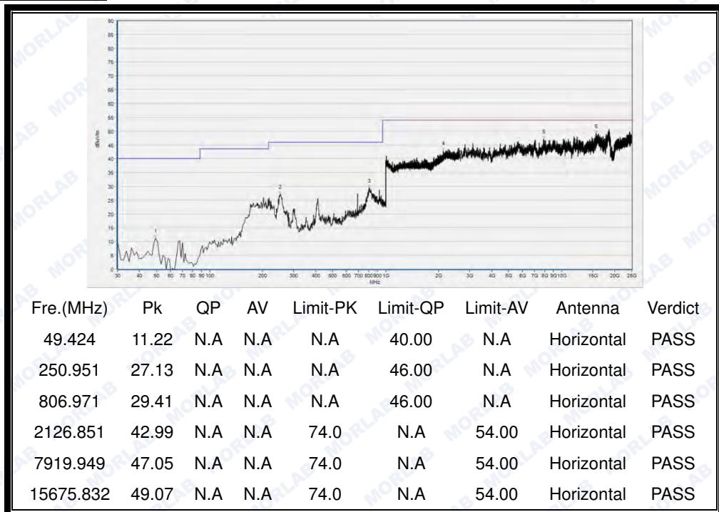
(30MHz to 25GHz, Antenna Horizontal @8-DPSK, channel 0)
