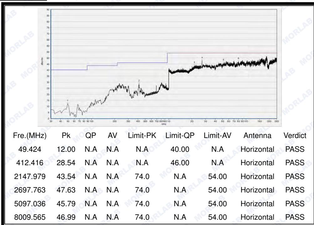
(30MHz to 25GHz, Antenna Horizontal @ GFSK, channel 78)
