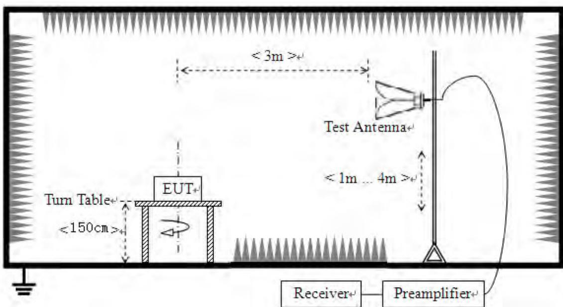
The Module is located in a 3m Semi-Anechoic Chamber; the antenna factors, cable loss and so on of the site as factors are calculated to correct the reading. During the measurement, the Bluetooth Module is activated and controlled by the Bluetooth Service Supplier (SS) via a Common Antenna, and is set to operate under hopping-on test mode transmitting 339 bytes DH5 packages at maximum power.
