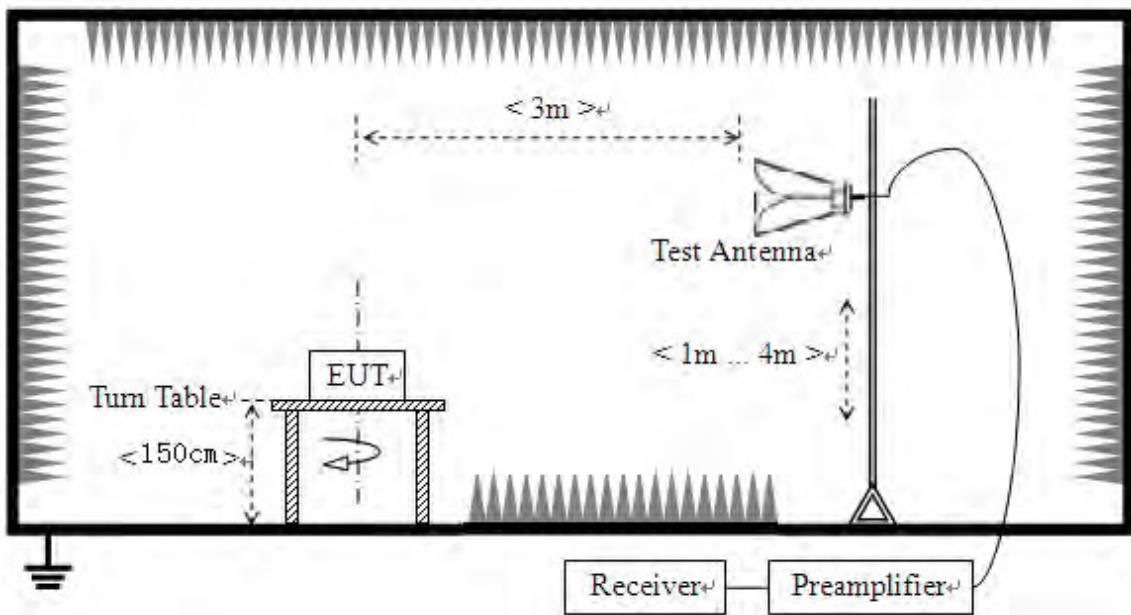
The test site semi-anechoic chamber has met the requirement of NSA tolerance 4dB according to the standards: ANSI C63.10 (2013). For radiated emissions below or equal to 1GHz, The EUT was set-up on insulator 80cm above the Ground Plane, For radiated emissions above 1GHz, The EUT was set-up on insulator 150cm above the Ground Plane. The set-up and test methods were according to ANSI C63.10.
