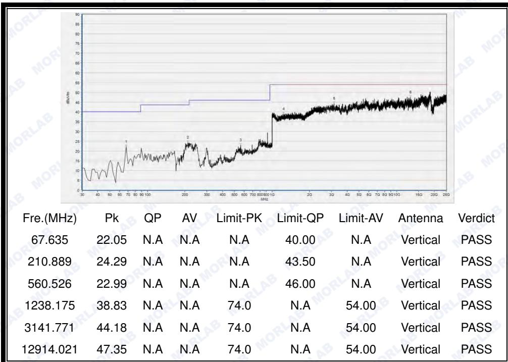
(30MHz to 25GHz, Antenna Vertical @ GFSK, channel 39)
