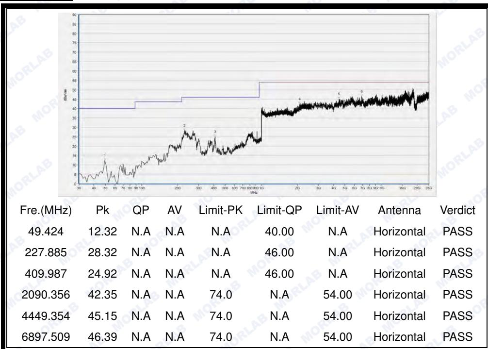
(30MHz to 25GHz, Antenna Horizontal @ GFSK, channel 39)
