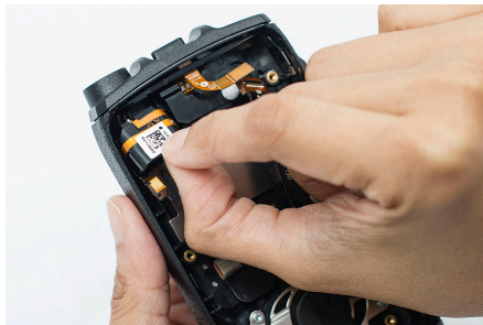
Figure 23: Detaching the Internal Antenna Module Assembly
