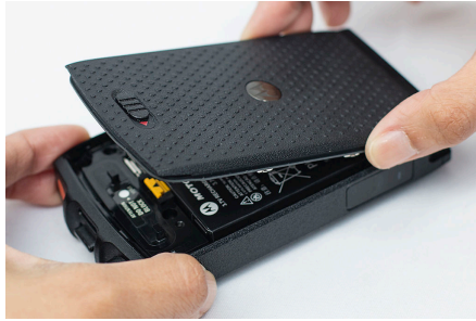
Figure 50: Attaching the Battery Cover
