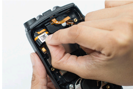
Figure 39: Installing the Internal Antenna Module Assembly
