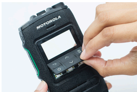
Figure 30: Removing the Front Keypad
