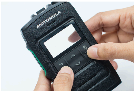
Figure 31: Inserting the Front Keypad
