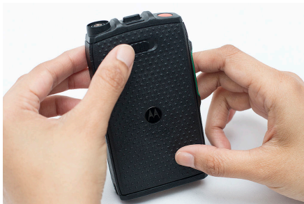
Figure 14: Unlocking the Battery Cover
