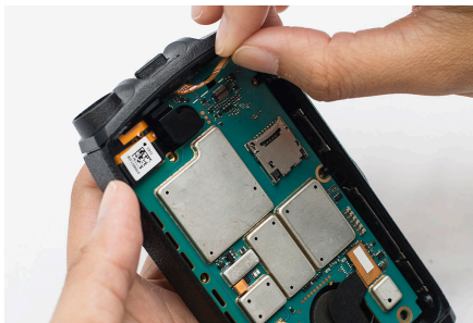
Figure 20: Detaching the Top Flex Connector
