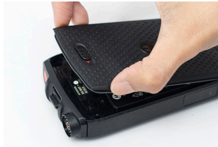
Figure 15: Removing the Battery Cover
