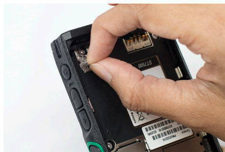
Figure 17: Removing the Tamper Label
