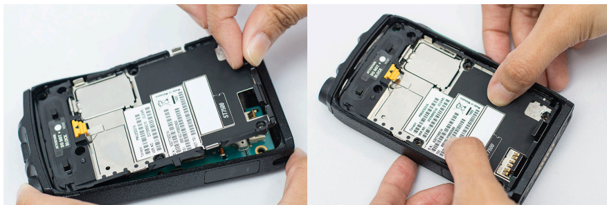
Figure 45: Installing the Back Housing
