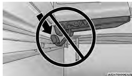
Improper Clamp Position
