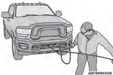
Pulling Synthetic Rope Under Tension
