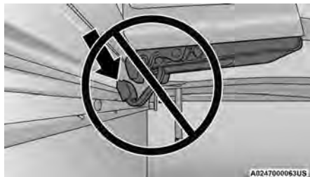
Improper Clamp Position
