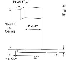
30" Models Require a 30"-Wide Opening \*The supplied duct cover fits 7'-5" to 9'-3" ceiling heights (10' with optional high ceiling kit JX10DC73)
