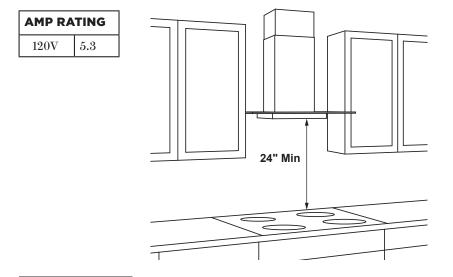
The vent hood must be installed 24" min. above the cooking surface. For optimal performance, installing the hood more than 36" above the cooking surface is not recommended. The hood installation height above the cooking surface depends upon ceiling height. The telescopic duct cover conceals the ductwork running from the top of the hood to the ceiling.
