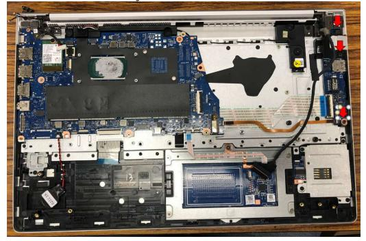
3.26 Use screwdriver to release man board, daughter board, and cable holder frame #1 screw 4 PCS
