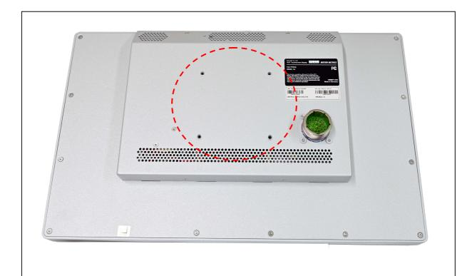
Figure 6: VESA Mounting on the rear side (MS-DSP15-100)
