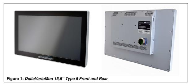
The integrated LCD TFT graphic module has a resolution of  $1.920 \times 1.080$  dot. The maximum brightness is  $1.200 \text{cd/m}^2$ . The brightness can be adjusted by DDC/CI signal which is integrated in the DVI Signal path from 0% to 100%. The additional integrated light sensor, automatically adjusts the screen brightness based by ambient light. The control is performed by a microcontroller, where the hysteresis- parameters are stored accordingly.
