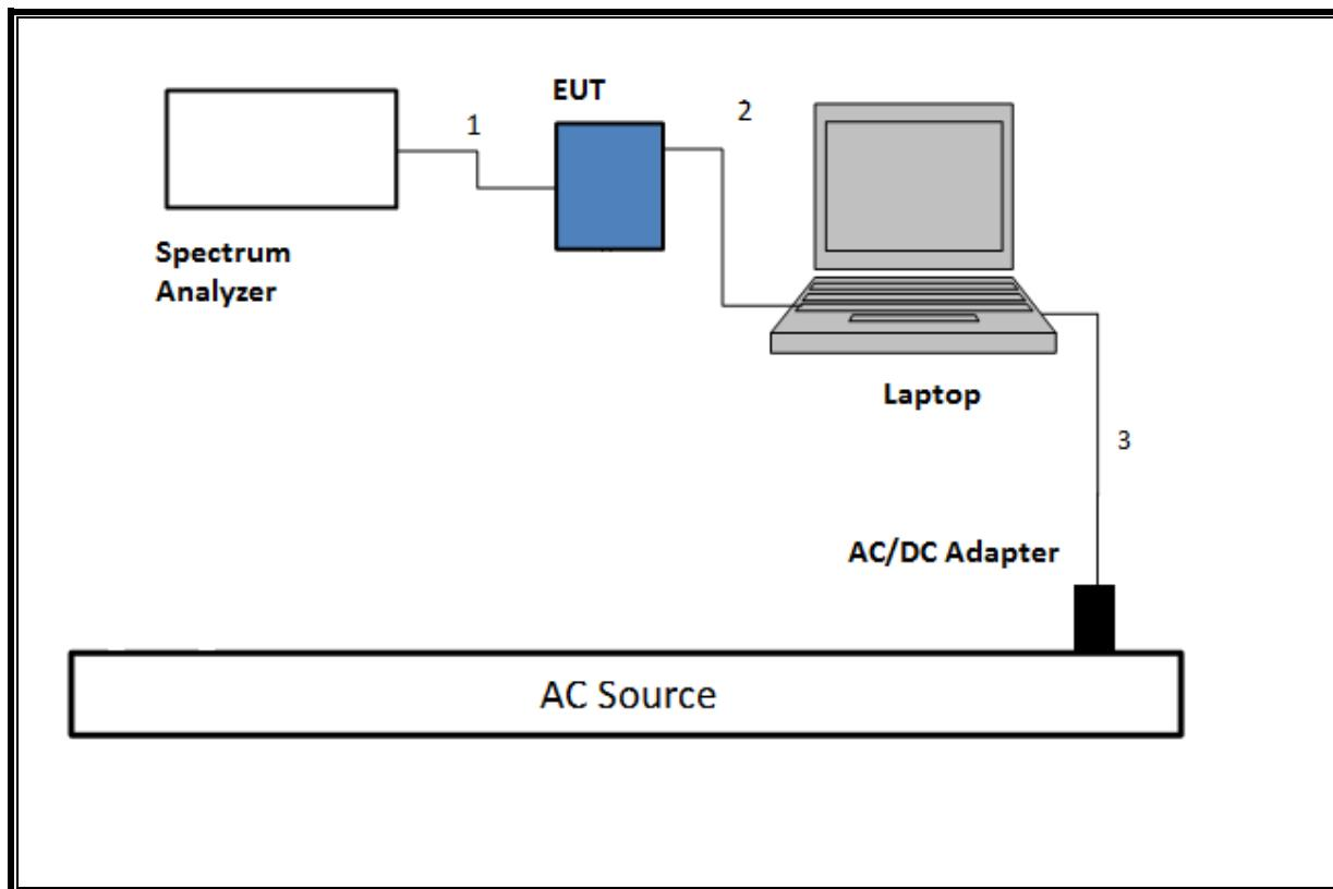
**SETUP DIAGRAM FOR RADIATED TESTS Above 1GHz**
