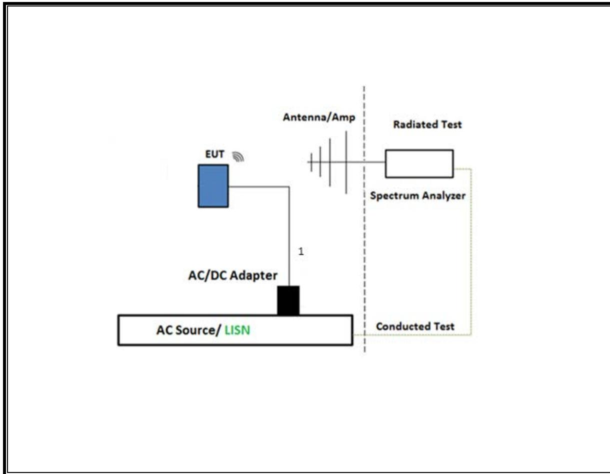
**TEST SETUP- AC LINE CONDUCTED: LAPTOP CONFIGURATION**
