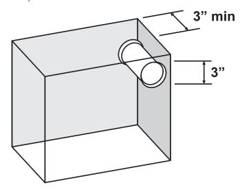
NOTE- When using a port you must leave a gap at least equal to the shortest measurement of the port between the rear of the enclosure and the port.
